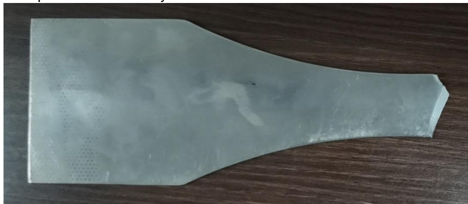
Figure 10-Typical macroscopic fracture of specimen
