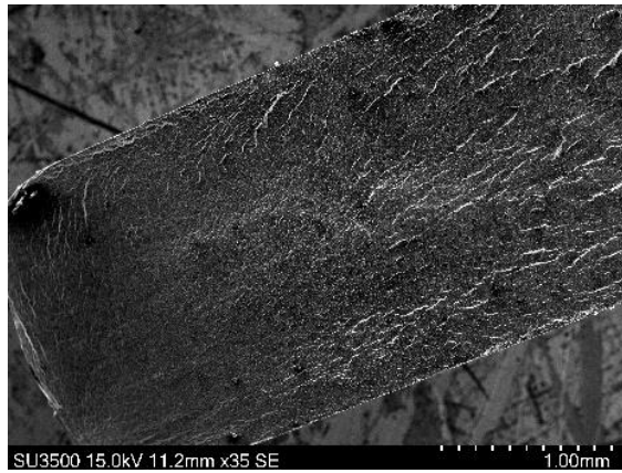
(a) Crack initiation end of the specimen
