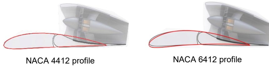
figure 5: Approximation of the wing profile selecting NACA 4412 profile, [16]
