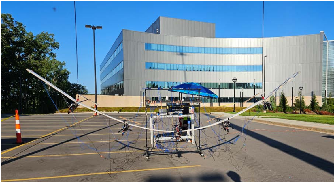
Figure 13 – The X-HALE suspended in the outboard configuration during the free-free GVT, connected to the bungee cords dropped from the crane.
