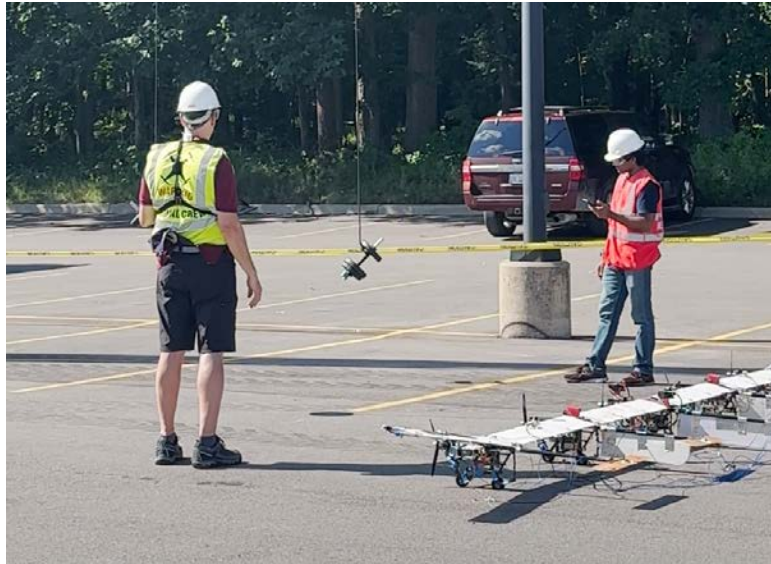
Figure 16 – The calibrated mass (dumbbell suspended from bungee cord, middle of the image) used to measure the bungee plunge frequency.
