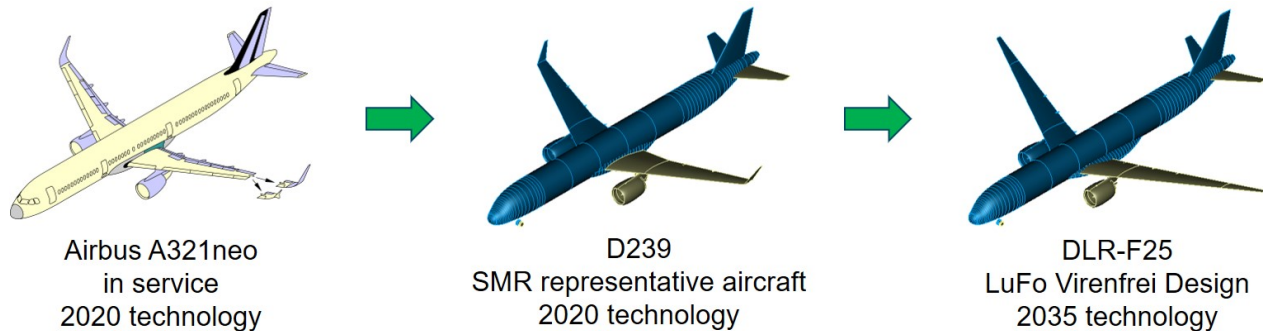
Figure 14 – Aircraft design process from the A321neo reference aircraft [23] to the D239 as the SMR representative aircraft to the DLR-F25 configuration.
