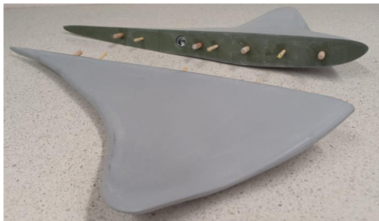
Fig. 19 - Interchangeable wings (aeroshape NM3).
