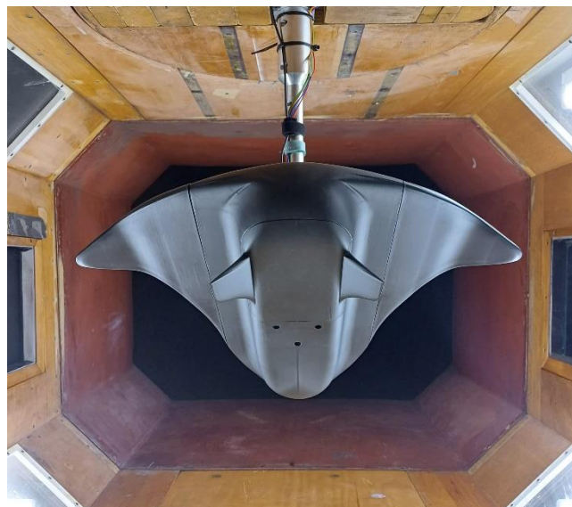
Fig. 26 – Aeroshape model NM3 installed at University of Sydney's 4x3ft WT.
