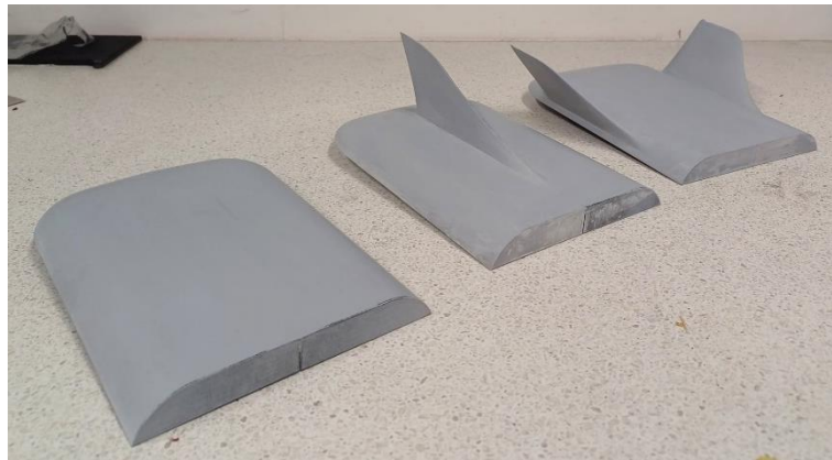
Fig. 18 - Interchangeable tails refined with putty spray and sanded.
