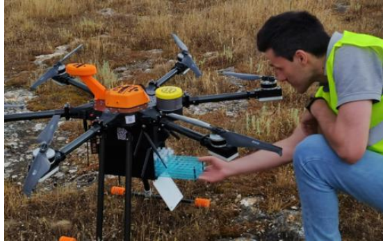
Figure 18: Techno Sky UAS used for BVLOS last mile delivery operation
