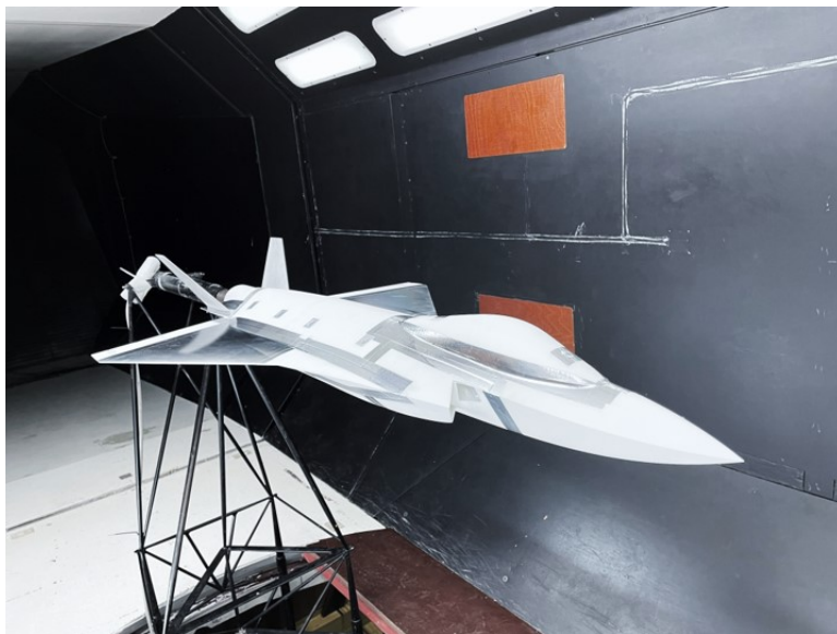
Figure 1 – Saab FCAS concept fighter in the L-2000 Wind tunnel at KTH.
