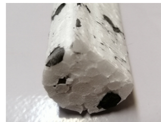
(b) Defect in foam cut out
