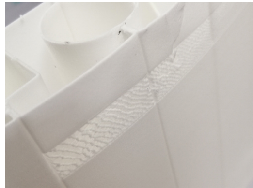
(b) Too thin walls
