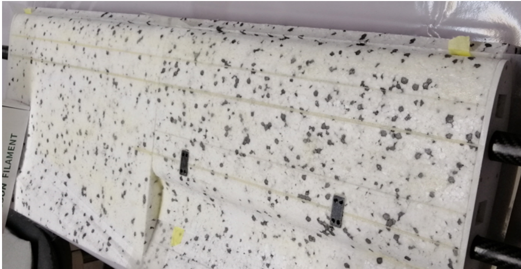
Figure 10 – Glued foam sections with the filling of cotton flocks
