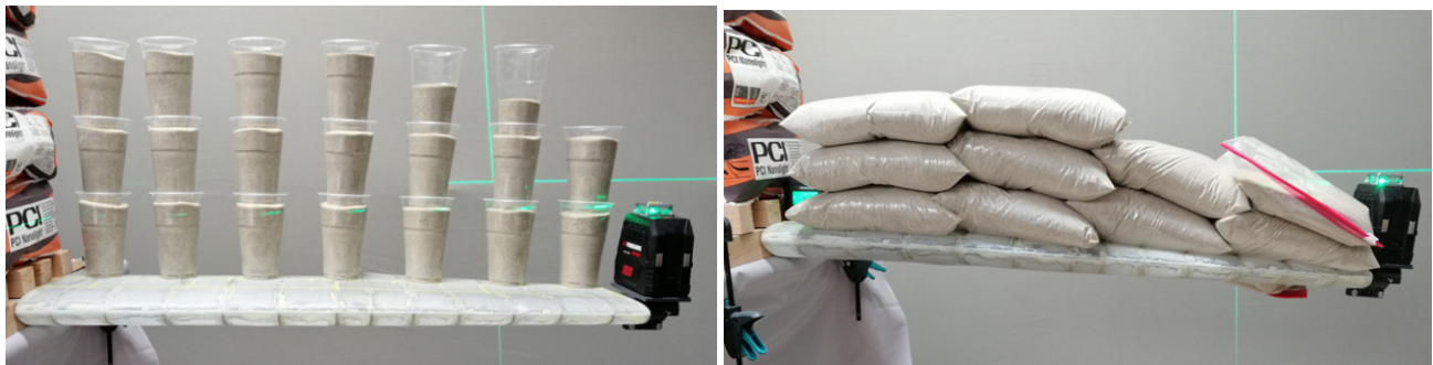
(a) Load distribution according to lift distribution
