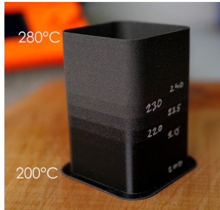
Figure 5 – Temperature tower with colorfabb's LW-PLA [19]
