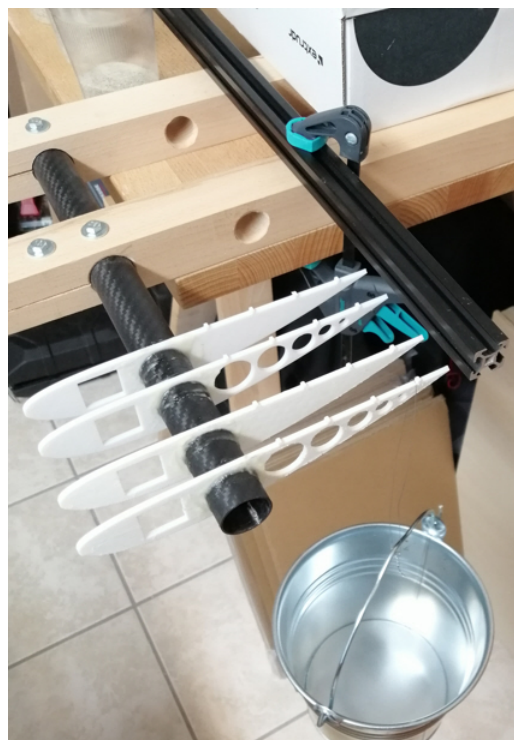
Figure 14 – test setup for ribs loadtests
