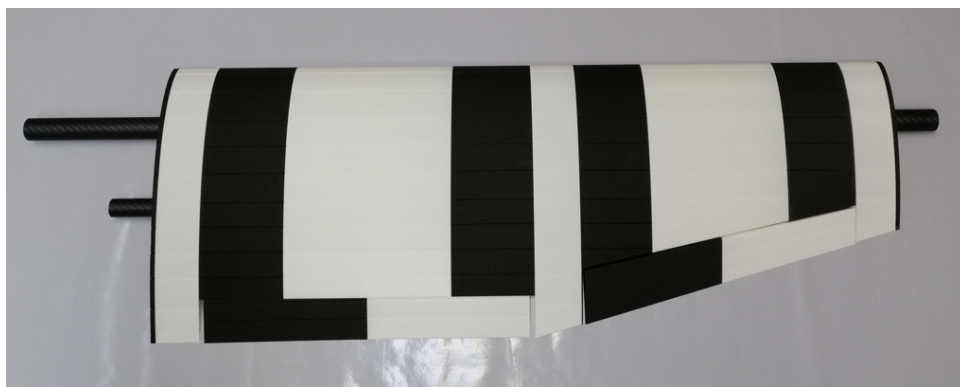
Figure 20 – Printed Section of M3 wing, flap and aileron
