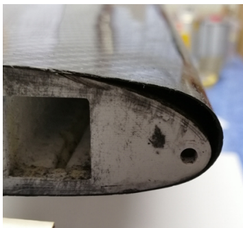
(a) Lifted leading edge in pretest
