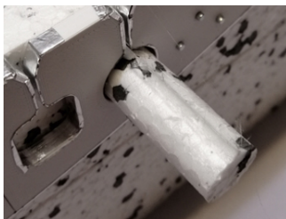
(a) Foam removal after cut
