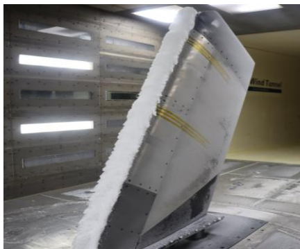
Figure 1 –The wing's leading edge's ice shape at a 30-degree sweep angle
