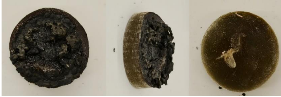
Fig. 9 – Photo of an example of a sample after ablation testing with 5% MMT.
