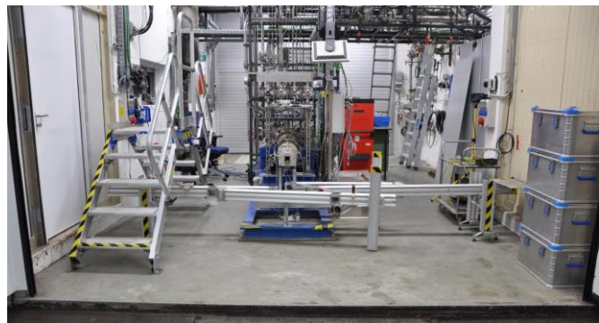
Figure 1. Chemical air vitiator test bench M11.1.
