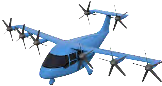
Figure 7 – The VTOL concept vehicle by Whiteside et al. [17] in its cruise configuration.
