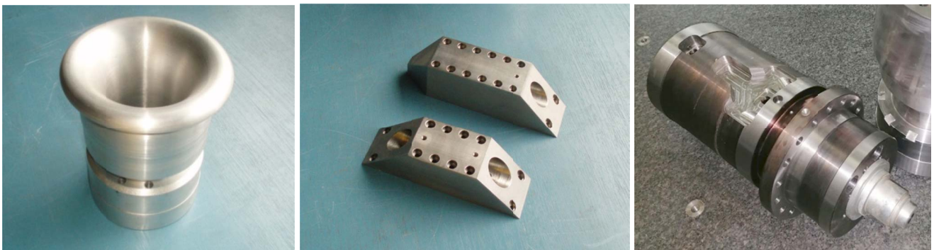
Figure 6 – Some components produced for the modified flow cell: Left: the bellmouth inlet for calibration; Middle: holders for cable conduit; Right: unfinished drive module and support flange
