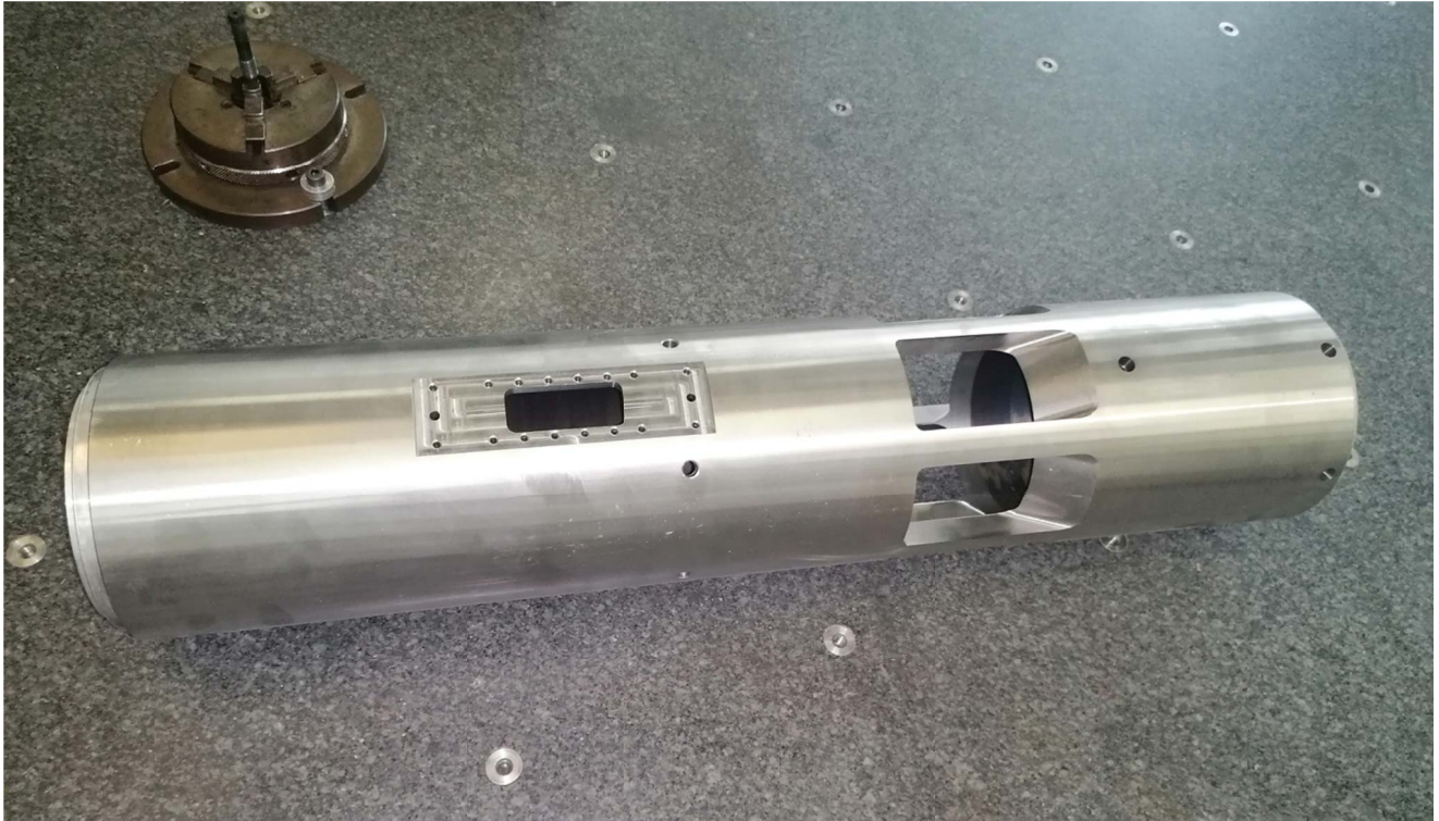
Figure 3 – New shell of the flow cell device being prepared for CMM control in VTI workshop
