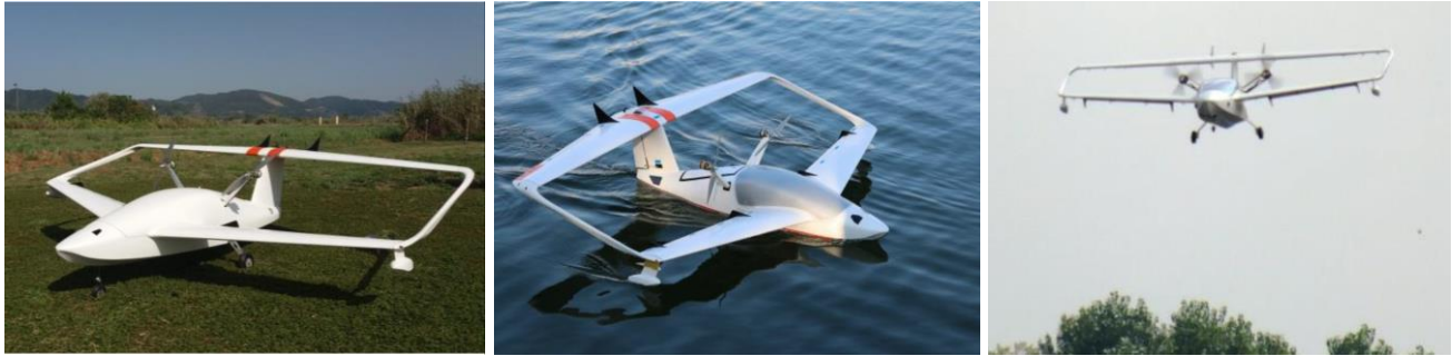
Figure 32. Scaled flying model in ground (left), in water (centre), and in flight (right)
