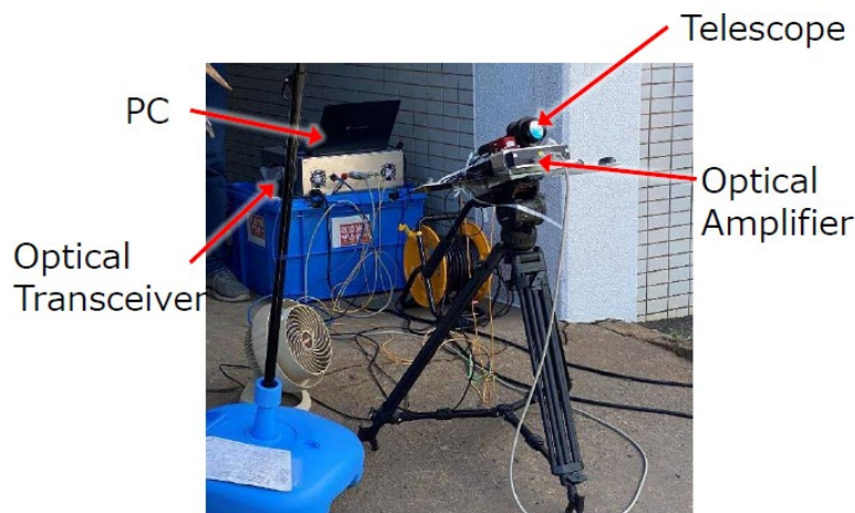
Figure 5 – Prototype polarization lidar.
