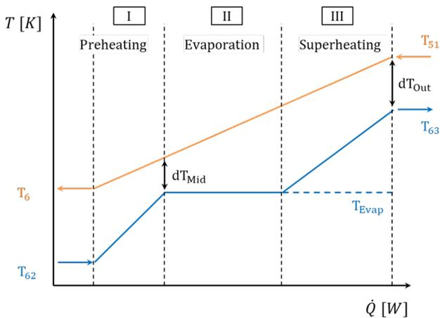
Figure 4 – Evaporator Model
