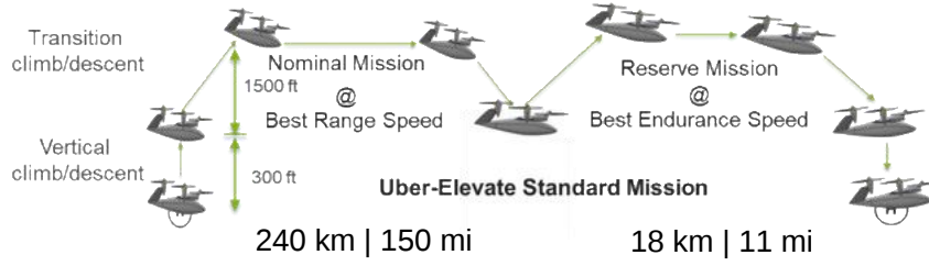
Figure 3. Nominal Mission consisting of a vertical climb and hover, and a forward flight segment consisting of a climb and 100-mile cruise.
