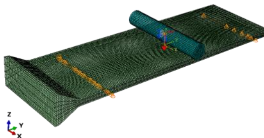
Figure 8 - Solid FEM model of 3-point bending test of 2.5D test element 7822 with single foot.
