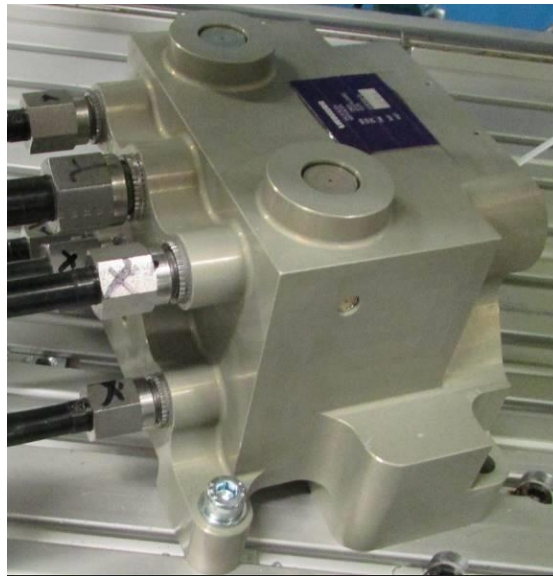
Figure 13 - ESTER TRL 6 valve block
