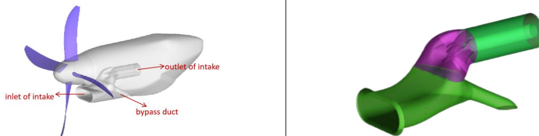
Figure 2 -A typical turboprop inlet with a bypass duct.
