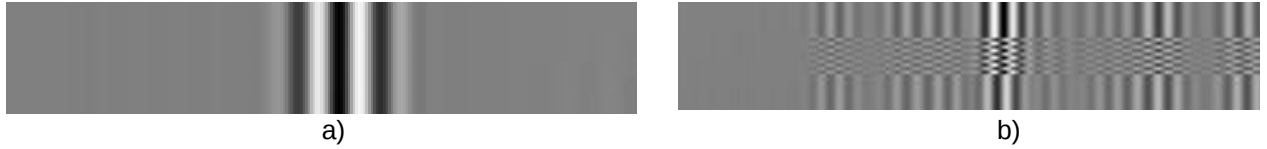
Fig. 6. RGB transformed signal: a) healthy path – b) damaged path.
