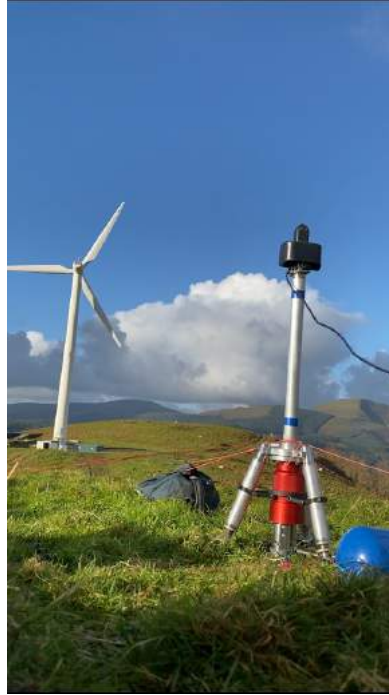
Figure 1: SnapShot autonomous nanodrone on its launcher, set-up downstream of the wind turbine prior to flight test
