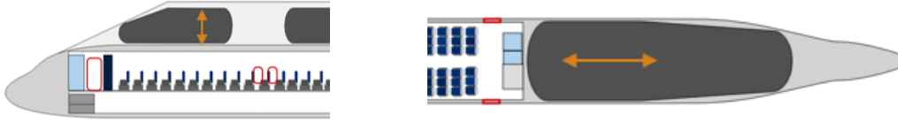
Figure 15 - Tank sizing options (Left: Over cabin tanks, right: full cross-section tanks)
