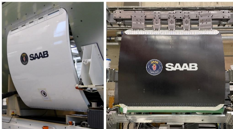
Figure 12 – The metallic TD4 cargo door installed in a single aisle demonstrator (left), composite TD5 cargo door mounted in the flexible assembly jig (right)
