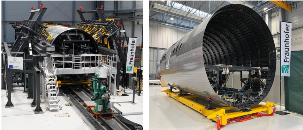
Figure 11 – Major Component Assembly facility at Fraunhofer (left) and MFFD after successful welding of longitudinal joints ready for shipping to ZAL
