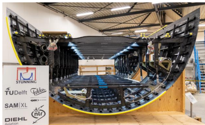
Figure 10 – MFFD lower shell module as delivered to the major component assembly facilities
