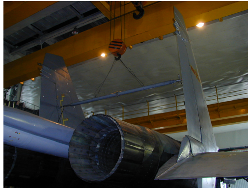
Figure 4-Twin vertical tail loading calibration test.
