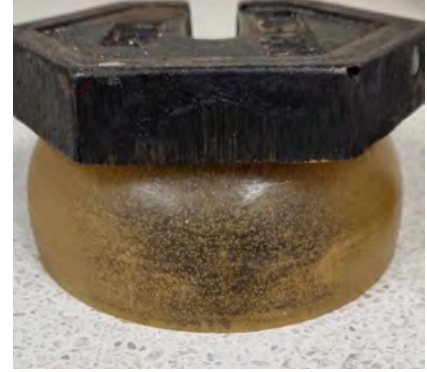
Figure 4 – Deformation of flexible hemisphere
