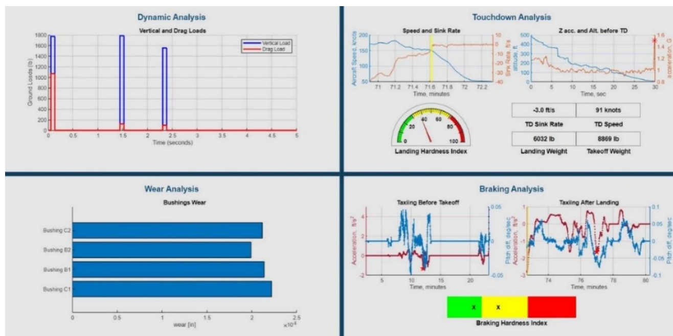
Figure 26 – Individual flight wear-analysis dashboard.
