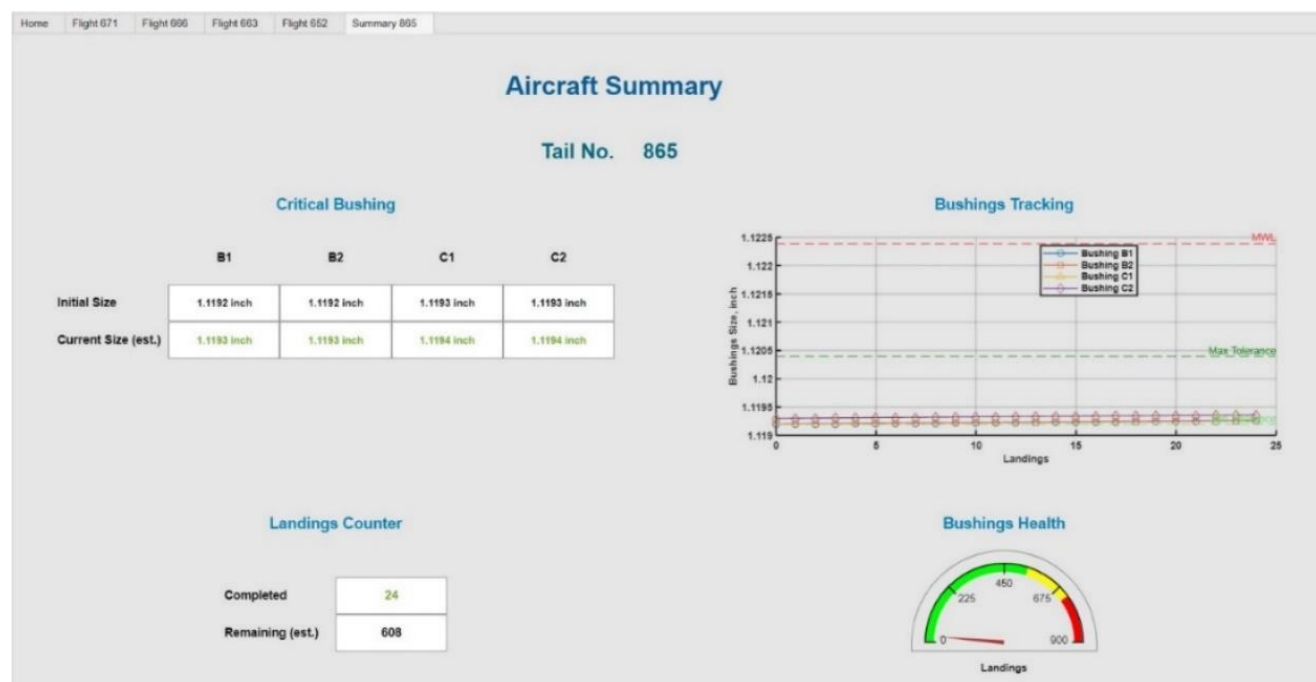
Figure 27 – Individual aircraft LS bushing health monitoring tab.
