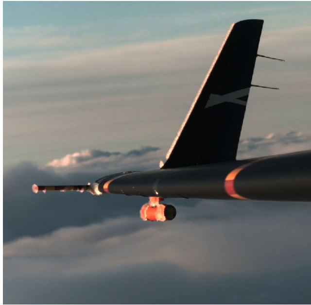
Figure 9 – Example of ice accretion on the Phenom 300 prototype outer right wing and winglet (white, glossy layer) during one flight of the SENS4ICE US icing flight test campaign; with permission, copyright Embraer
