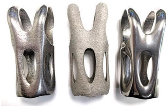
Figure 9: Typical surface finish of AM as-built material (Centre), with surface finishing. Surface after finishing on non-HIPed material (Left), and surface finishing after HIP (Right). [17]
