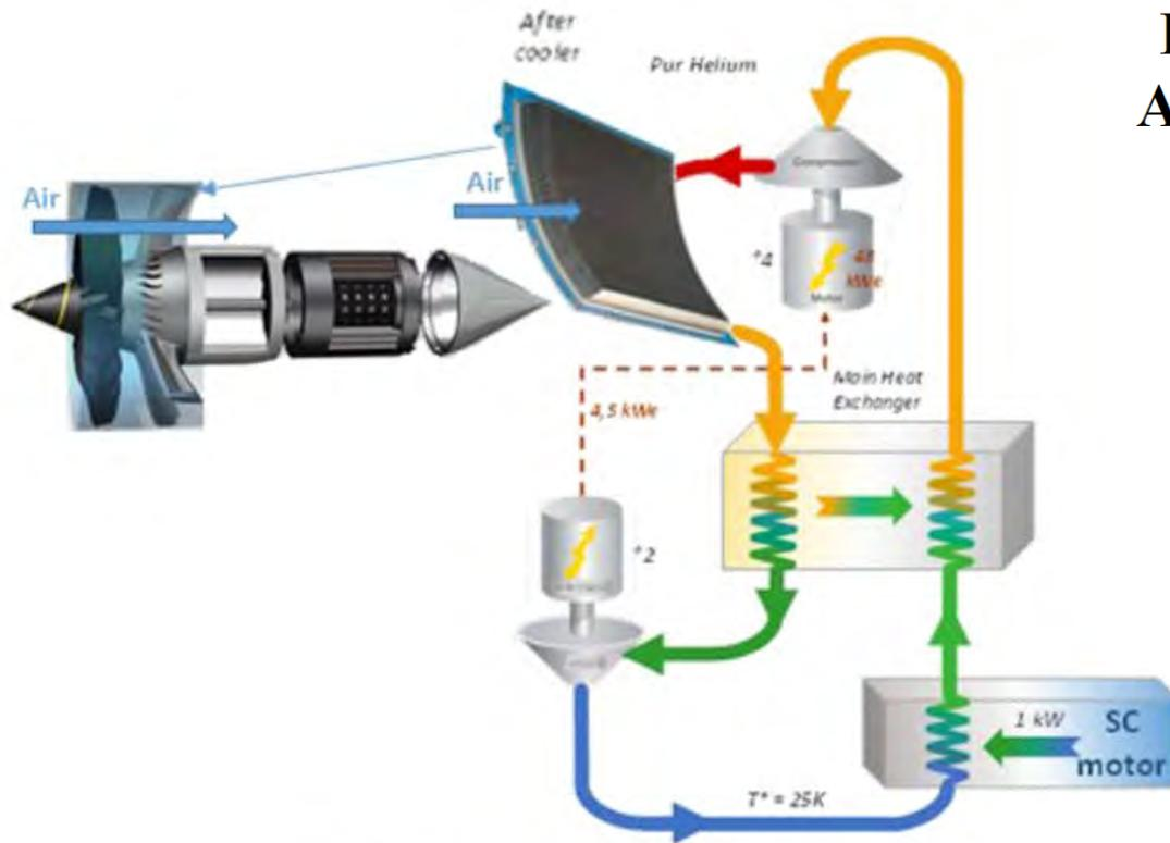
Figure 1: cryocooler cycle with air as hot sink
