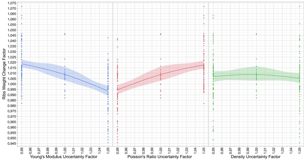
Figure 9 – Impact of wing structure material uncertainty factors on the overall wing weight
