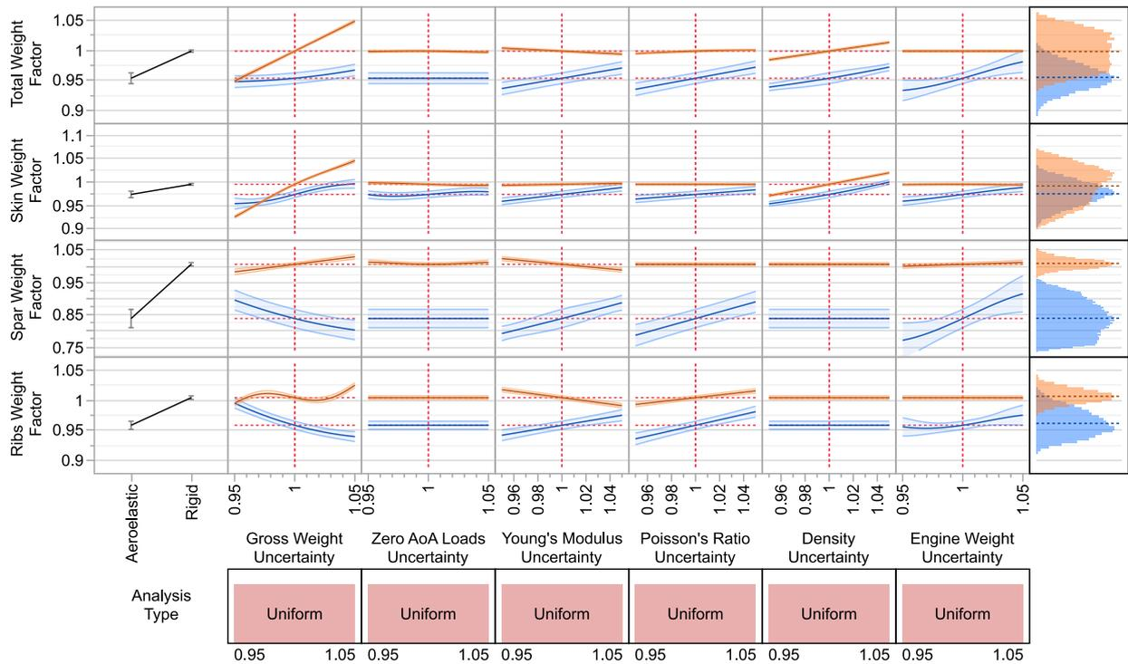
Figure 11 – Prediction profiler for parameter uncertainties (decoupled analysis in orange, aeroelastic analysis in blue)
