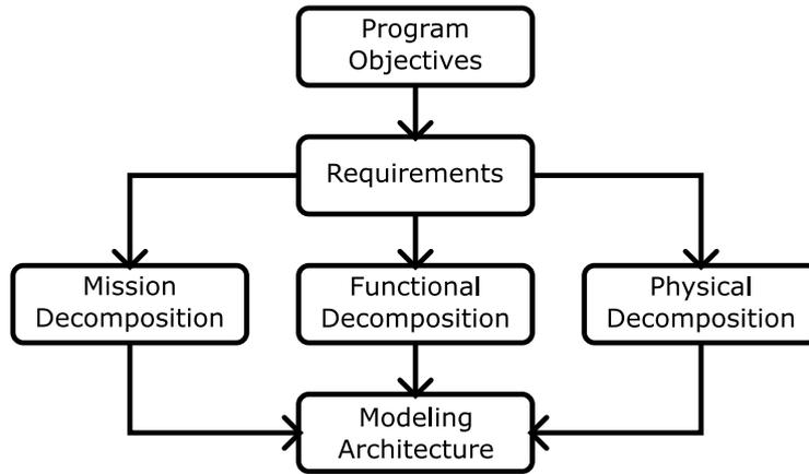
Figure 2 – System decompositions leading to modeling architecture
