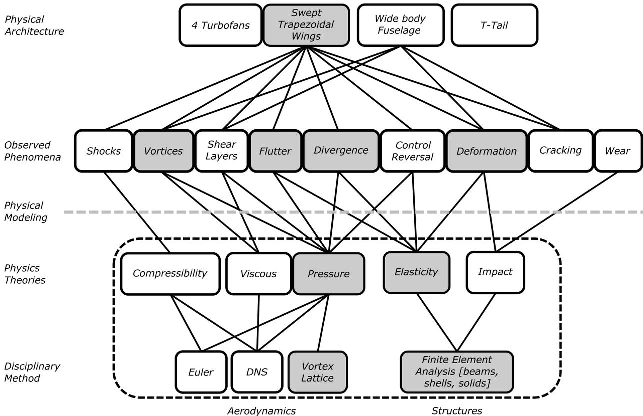
Figure 3 – Modeling architecture from an aerodynamics and structures perspective.
