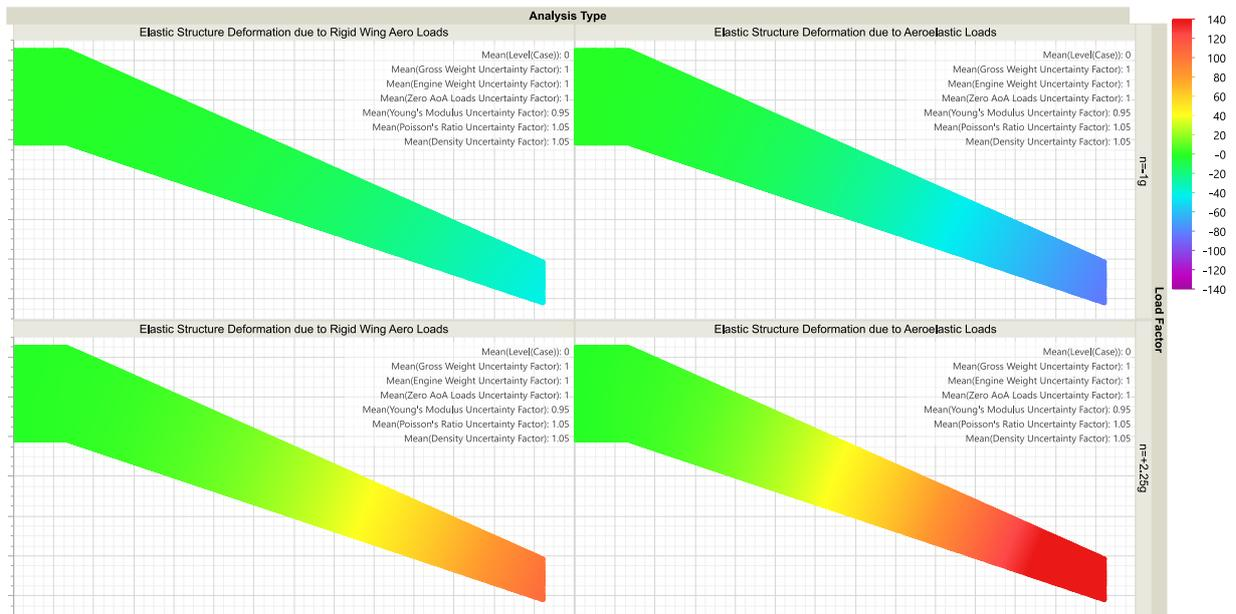
Figure 10 – Wing box deflection due to aerodynamic loads Top row: Load Factor = -1g, Bottom row: Load Factor = +2.25g. Left column: Decoupled Analysis, Right column: Coupled Analysis
