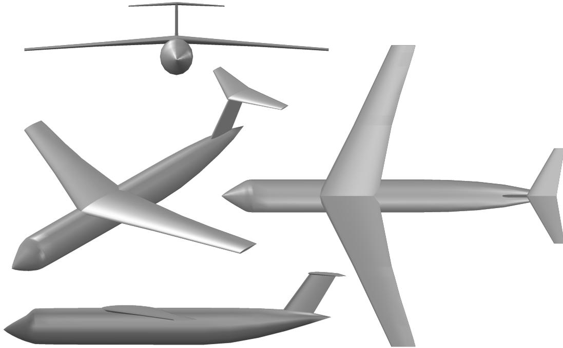
Figure 4 – OpenVSP model of the Lockheed C-5M
