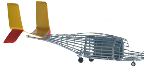
Figure 28 – Structural concept of fuselage with module installed
