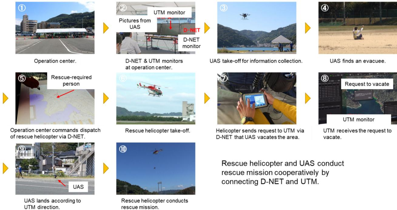
Fig. 9 Cooperative rescue mission of manned helicopter and UAS by connecting D-NET and UTM.
