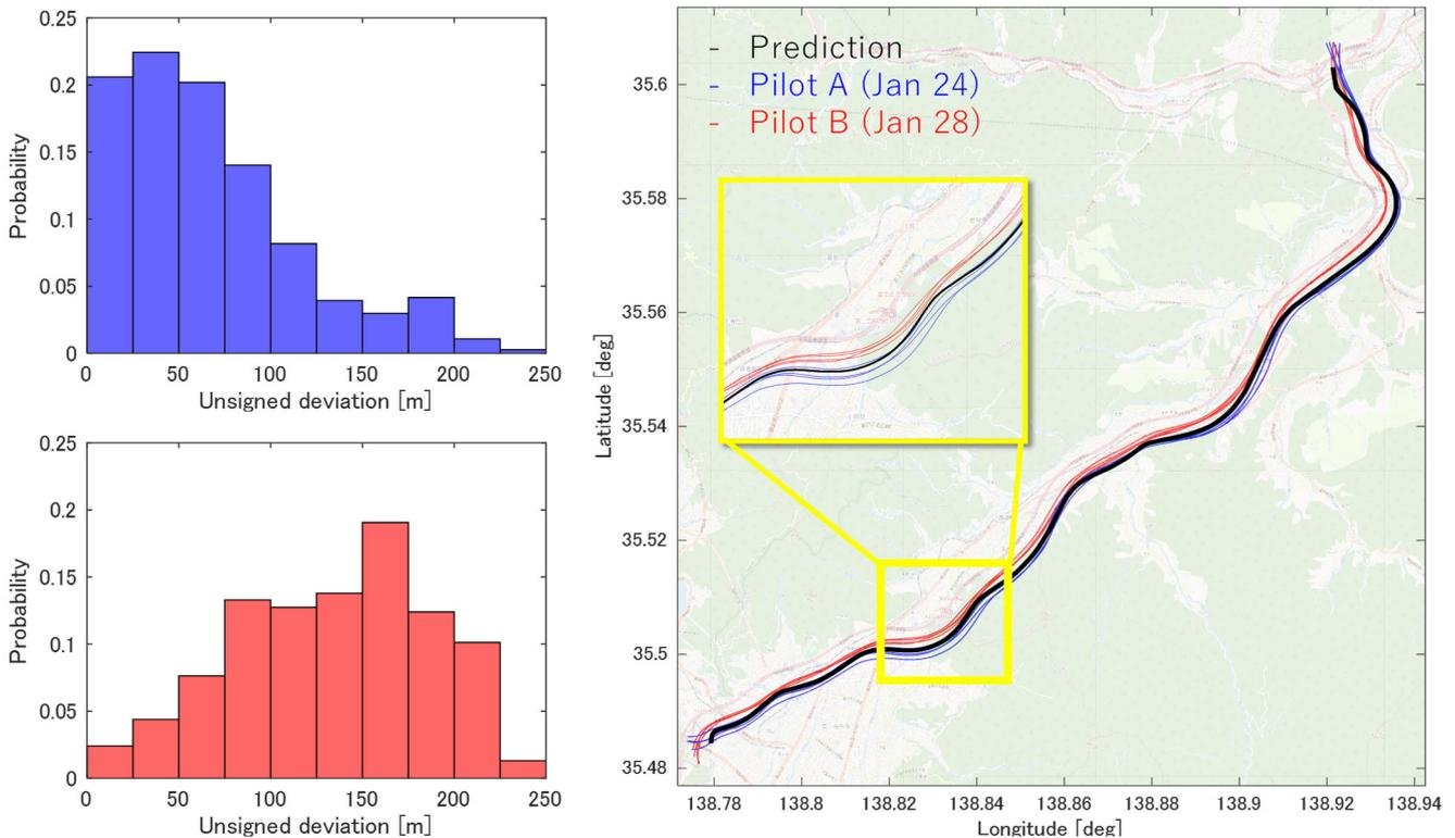
Fig. 7 Pilot's dependence and deviations from the predicted trajectory
