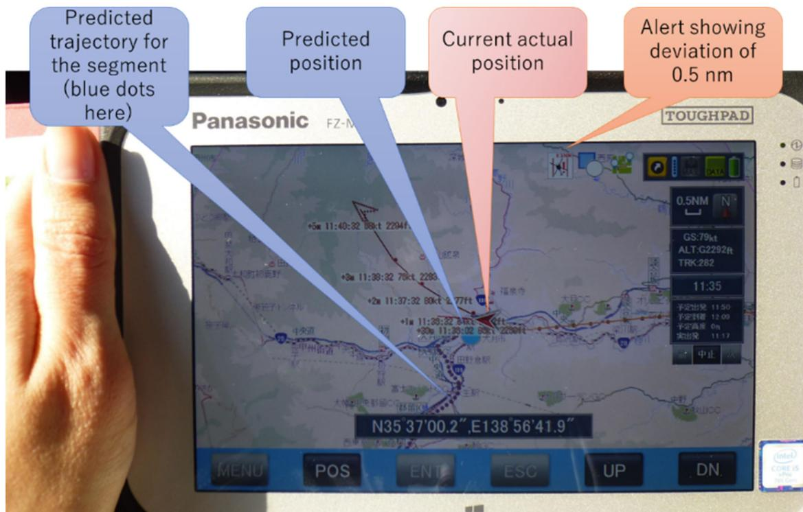
Fig. 8 D-NET onboard system showing the predicted and actual flight positions and deviation
