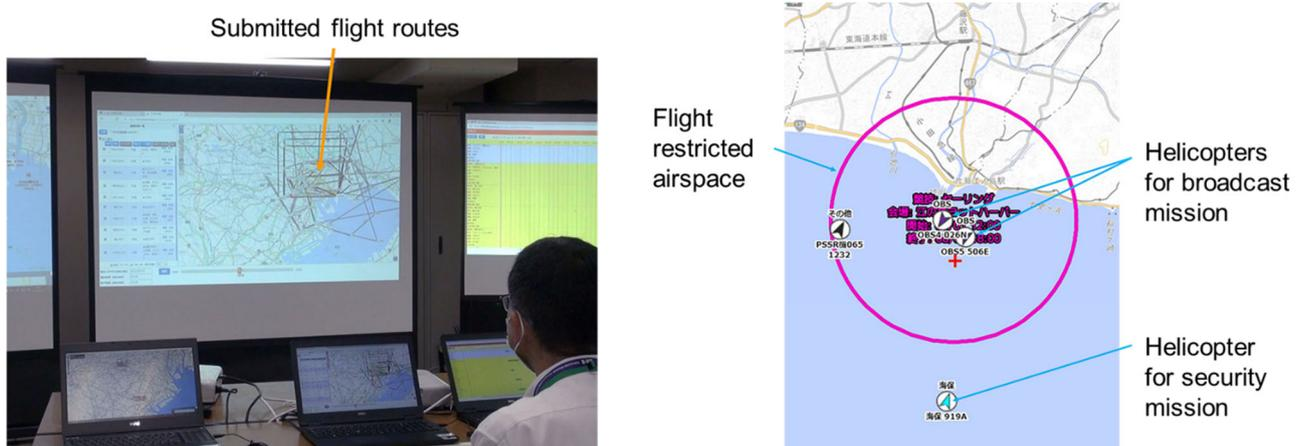
Fig. 5 Flight plan coordination in pre-flight phase (left) and aircraft monitoring in flight phase (right) using D-NET at Tokyo 2020 Olympic/Paralympic games.
