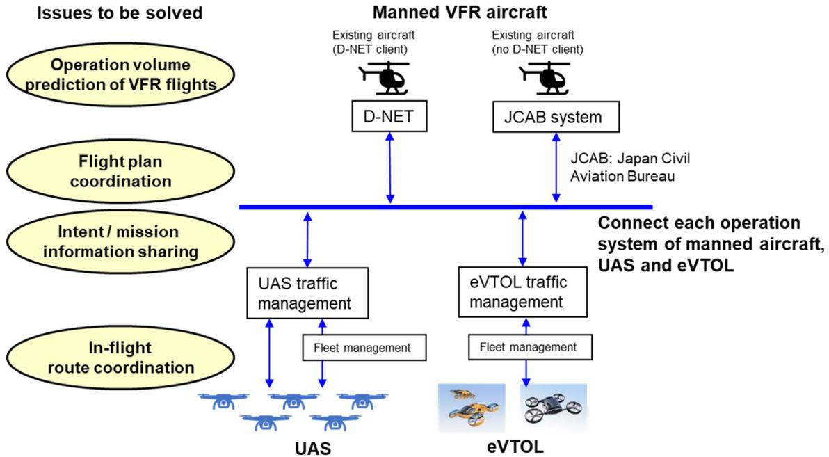
Fig. 6 Concept of integrated operation of manned aircraft, eVTOL and UAS.
