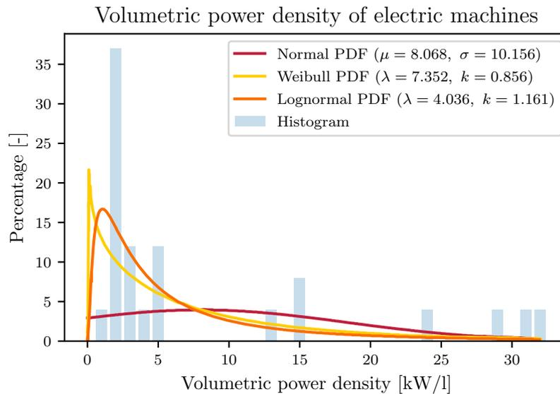
Figure 9 – Distributions of volumetric power density of current electrical machines
