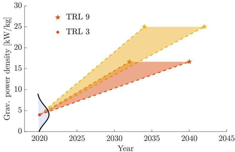
Figure 10 – Future uncertainty due to the specification of the current TRL using the example of gravimetric power density
