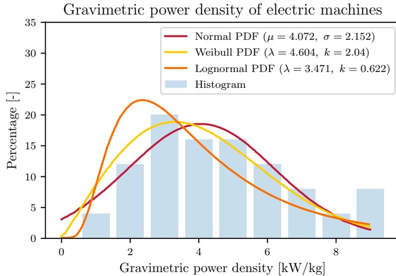
Figure 8 – Distributions of gravimetric power density of current electrical machines
