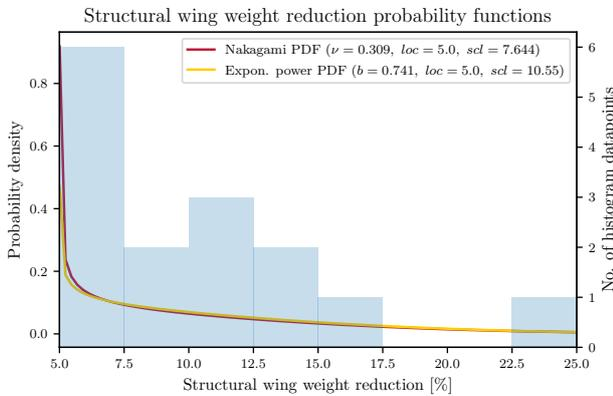
Figure 15 – Probability density function for structural weight reduction datapoints
