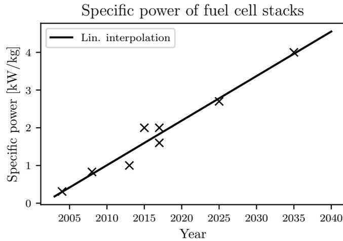
Figure 5 – Expected increase of the specific power of fuel cell stacks
