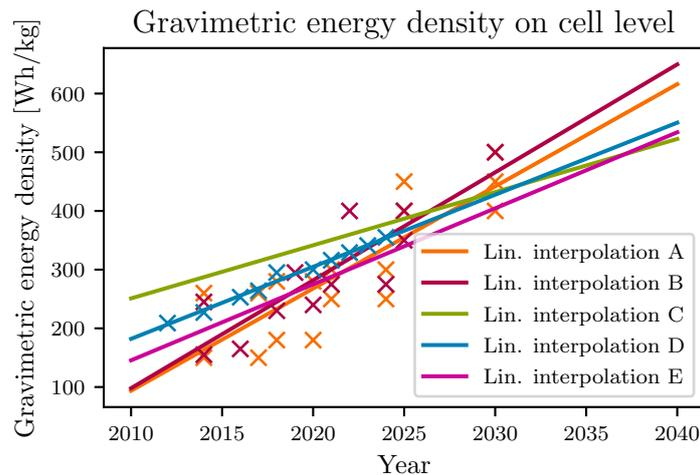
Figure 3 – Expected increase of the gravimetric energy density of lithium-based battery technologies
