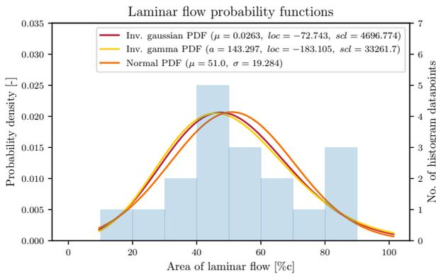
Figure 12 – Probability density functions for laminar flow control datapoints
