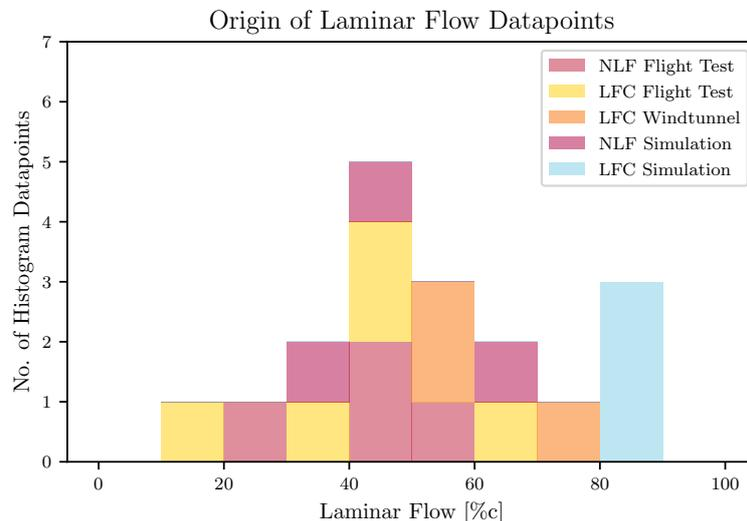
Figure 11 – Histogram and data type for laminar flow control datapoints
