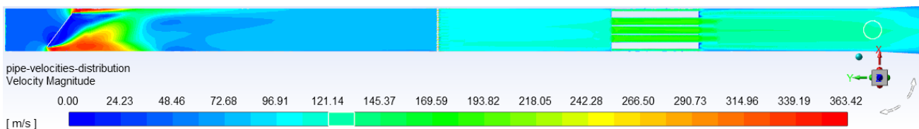
Figure 8 – Velocities distribution in pipe before pre-diffuser
