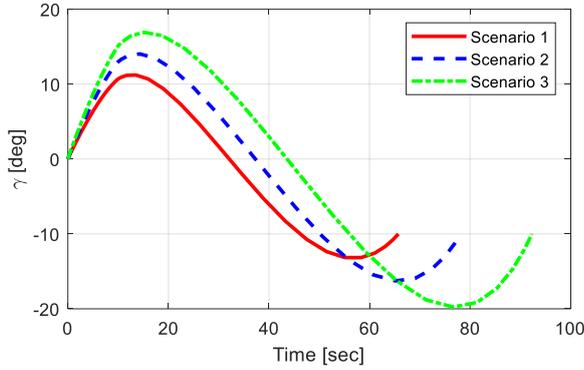
Figure 12 – Total angle-of-attack profiles with terminal heading angle.
