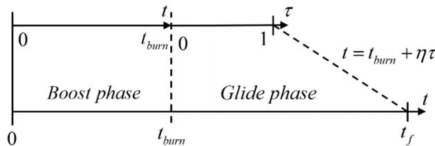
Figure 2 – Relationship between time and new independent variable.
