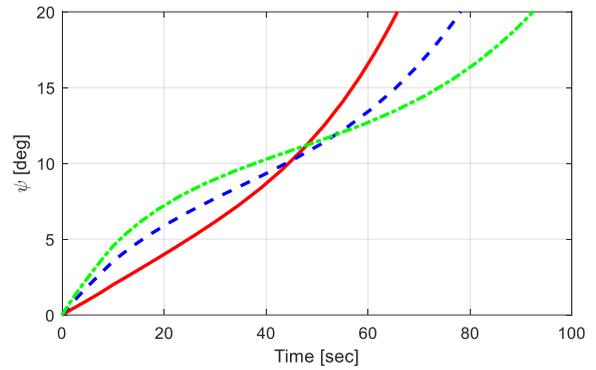
Figure 13 – Flight-path angle with terminal heading angle.
