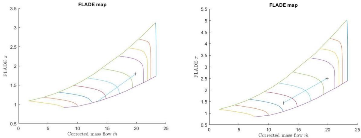
Figure 3: Left: FLADE design FPR=1.79 and Right: FLADE design FPR=2.0.
