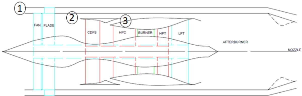
Figure 1: Schematic sketch for ACE engine architecture
