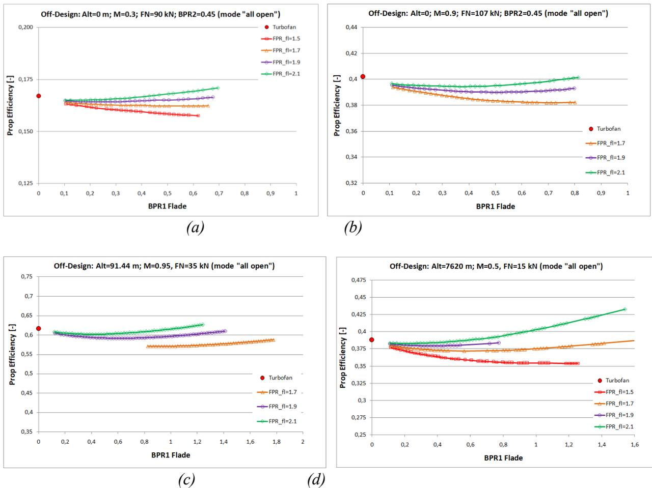
Figure 5: BPR1 Effect on the ACE propulsive efficiency for “all open” mode at the off-design conditions: (a) Case No 01; (b) Case No 02; (c) Case No 03; (d) Case No 04.
