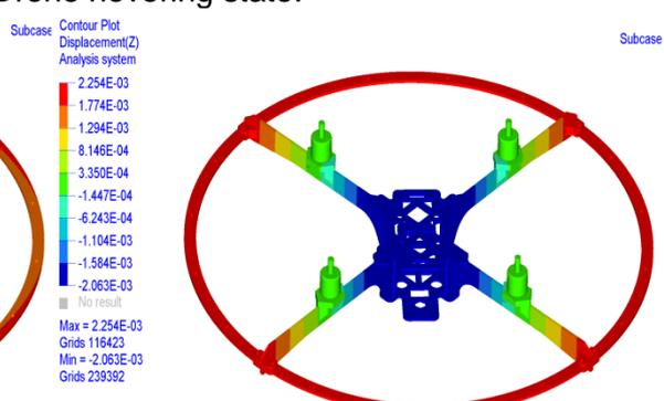
Figure 22 – Z-direction structural strain diagram.
