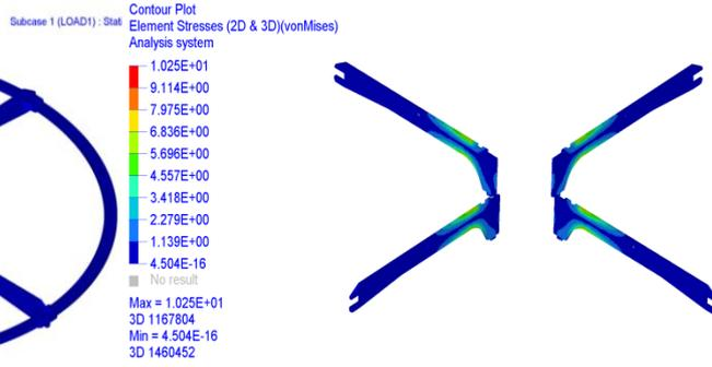
Figure 19 – Arm structure stress diagram.
