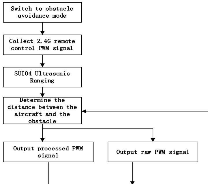
Figure 35 – Obstacle avoidance process.
