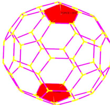
Figure 27 – The constraints and loads.
