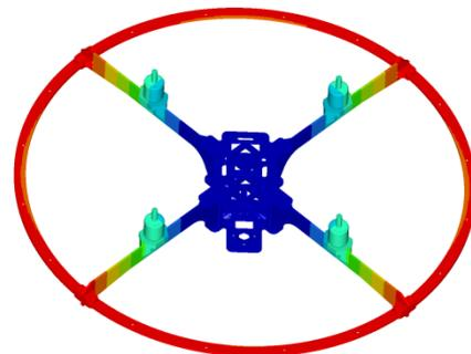
Figure 16 – Structural Strain Diagram.
