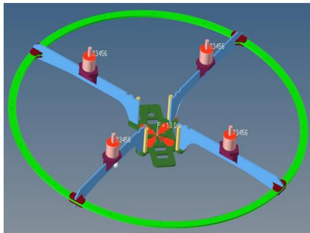
Figure 20 – Drone hovering state.
