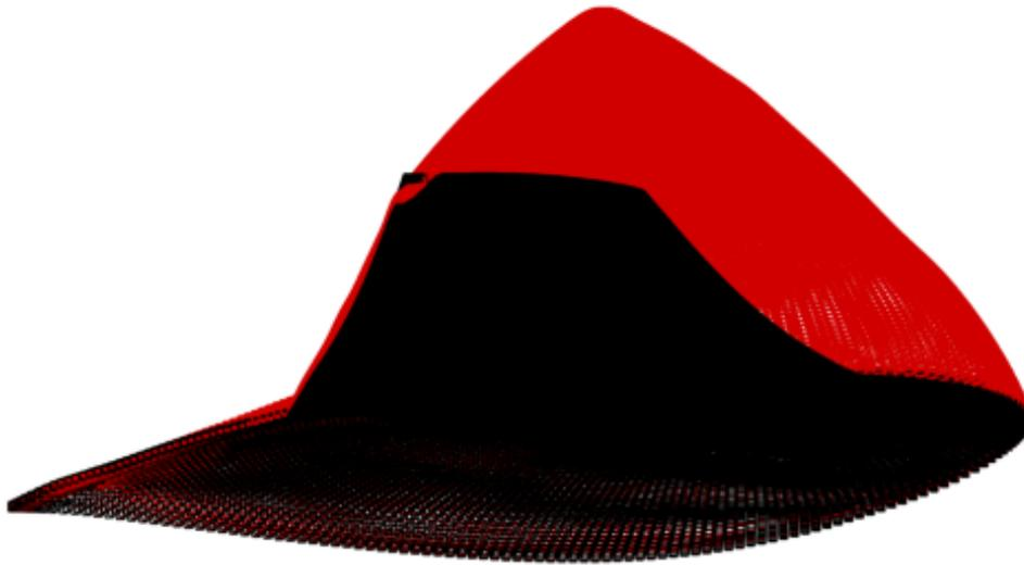
Figure 15 – Twist applied to the CRM wing. The wing in black indicates the original geometry and the red one is the modified wing.
