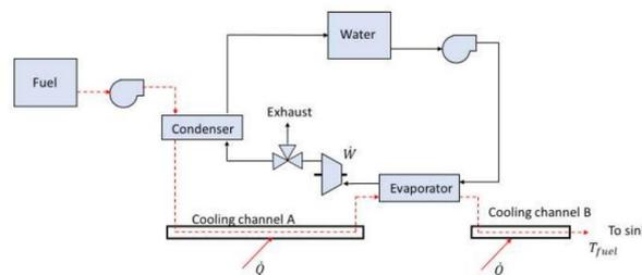
Figure.1. Rankine cycle TMS utilizing fuel as the working fluid [4]
