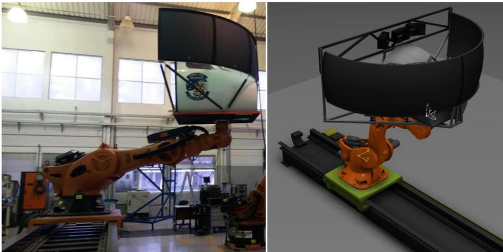
Figure 3. SIVOR flight simulator (cabin with embedded visual system on a robot arm).
