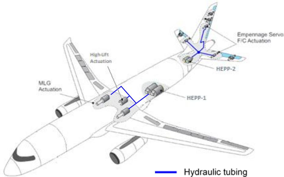
Figure 1 – Decentralized hydraulic power generation
