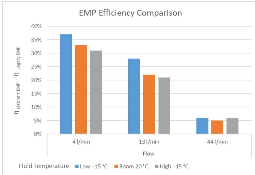
Figure 11 – EMP back-to-back test - Efficiency
