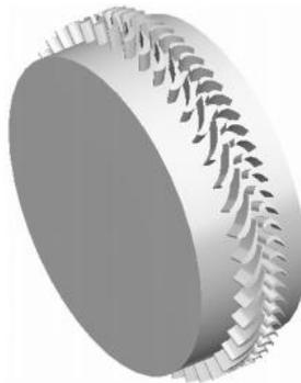
Figure 3 – 3D view of the LPOTP turbine first stage [21].
