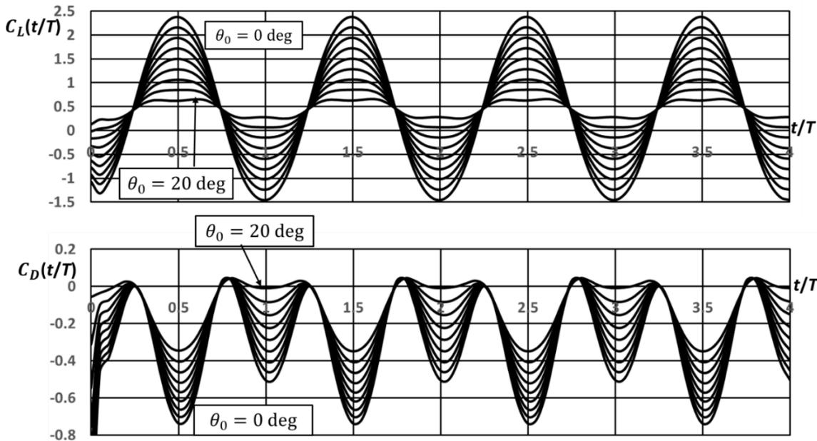
Figure 16 – Upper: Temporal lift coefficient  $C_L(t/T)$ . Lower: Temporal drag coefficient  $C_D(t/T)$ . Lifting line method of simplified configuration, for conditions listed in Table 1 and Table 2,  $St = 0.3343$ ,  $\theta_0 = 0(2.5)20$  deg,  $N = 80$ ,  $\frac{\Delta t}{T} = 0.05$ .
