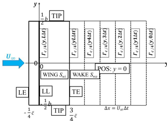
Figure 8 – Time-stepping procedure progressed to time  $t = L\Delta t$ ,  $L = 5$ .
