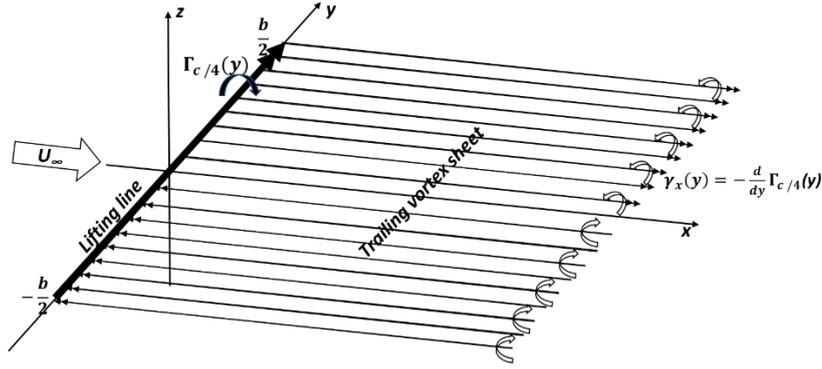
Figure 6 – Prandtl's lifting-line theory for incompressible potential flow about high-aspect ratio wing at angle of attack. Note that origin coordinate system is on lifting line.
