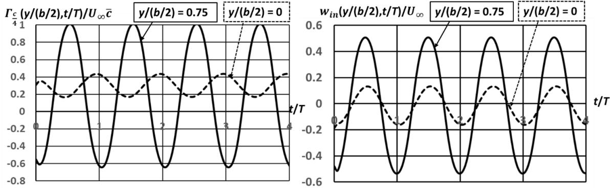
Figure 13 – Temporal evolution of circulation  $\Gamma_{c/4}(y, t)$  (left) and upwash  $w_{in}(y, t)$  (right) for simplified configuration, at root  $y = 0$  (dashed line) and near tip  $y = \frac{3b}{42}$  (solid line). Conditions listed in Table 1 and 2,  $\theta_0 = 10$  deg,  $N = 80$ ,  $\frac{\Delta t}{T} = 0.05$ . Plot contains results for four flapping cycles.
