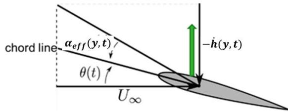
Figure 3 – Effective angle of attack  $\alpha_{eff}(y, t)$  due to plunging/pitching motion. Green arrow indicates direction of plunging motion. Angle of attack due to plunging motion equals  $\alpha_{plunge} = \arctan \left( \frac{-1}{U_\infty} \frac{\partial h(y, t)}{\partial t} \right)$ .
