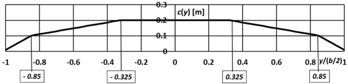
Figure 7 - Spanwise distribution of chord  $c(y/0.5b)$  of simplified planform of wind-tunnel model Robird.
