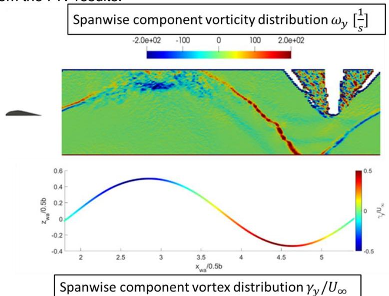
Figure 20 – Top: Spanwise ( $y$ -)component of vorticity measured for  $U_\infty = 6$  m/s (see Table 3) on plane at  $y = 220$  mm, which is approximately at half semi-span of wing. Bottom: similar cross-section approximated wake vortex sheet with strength spanwise component wake vortex distribution indicated by colour.
