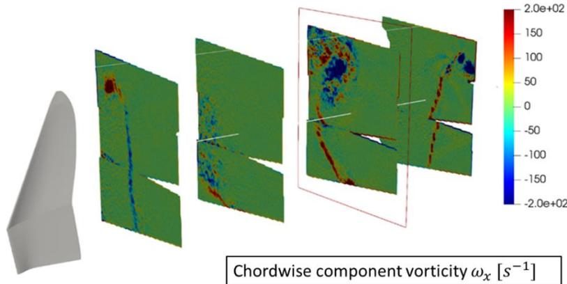
Figure 21 - Tip vortex for different moments in flapping cycle for  $U_\infty = 6$  m/s (see Table 3), visualized through chordwise component vorticity  $\omega_x$ . Cutting planes: from right to left: upstroke, halfway upstroke, end of upstroke and downstroke. Adapted from [21].
