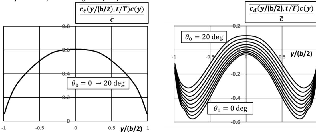
Figure 15 – Left: Spanwise distribution cycle-averaged section wing loading  $\overline{c_\ell(y/(b/2), t/T)c(y)/\bar{c}}$ . Right: Spanwise distribution cycle-averaged section axial loading  $\overline{c_d(y/(b/2), t/T)c(y)/\bar{c}}$ . Lifting line method of simplified configuration, for conditions listed in Table 1 and Table 2,  $St = 0.3343$ ,  $\theta_0 = 0(2.5)20$  deg,  $N = 80$ ,  $\frac{\Delta t}{T} = 0.05$ .
