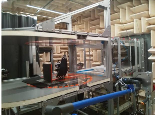
Figure 9 - Full-scale Robird wing (black with checker pattern in root and tip region) mounted in open section of UT aeroacoustics wind tunnel. Also visible: calibration plate, blue articulated optic arm; two Phantom V611 high-speed cameras. Flow is from right to left.
