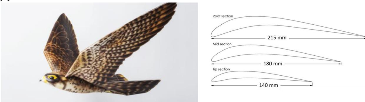
Figure 1 – Robird [1]: Design robotic bird based on Peregrine falcon (left). Typical airfoil sections wing Robird. (right).
