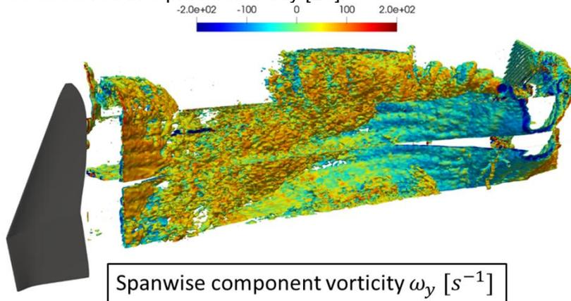
Figure 19 - Visualisation flow measurements for  $U_\infty = 6$  m/s (see Table 3), facing pressure side of wing. Shown are iso-volumes of vorticity magnitude  $|\vec{\omega}| \in = [100,300]$  [1/s] with intervals of 50 [1/s]. The contours are coloured with value of spanwise vorticity. Note that the wake is sinusoidal and represents a single period of the wing flapping cycle: starting with the upstroke at the far right, moving through zero-position in the middle of the wake.
