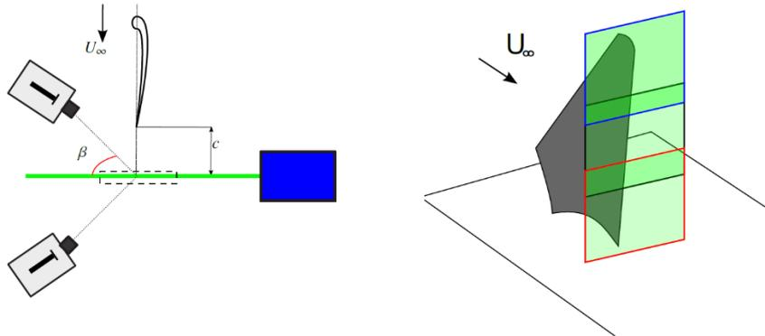
Figure - 10 Schematic of setup (a) top view: orientation of laser sheets, laser optics (blue box) and cameras (two grey objects at left side). (b) oblique view: three measurement volumes used, one at wing tip in blue, one at mid-wing section in black and one at root in red.
