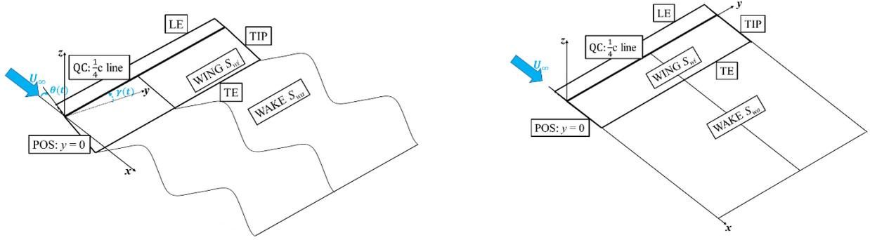
Figure 5 – Starboard side flapping-wing configuration at certain moment in cycle. Left: Flapping-pitching thin wing with wavy wake. Right: Stationary reference surface for application unsteady transpiration boundary conditions on wing and wake. Note that origin is on QC.
