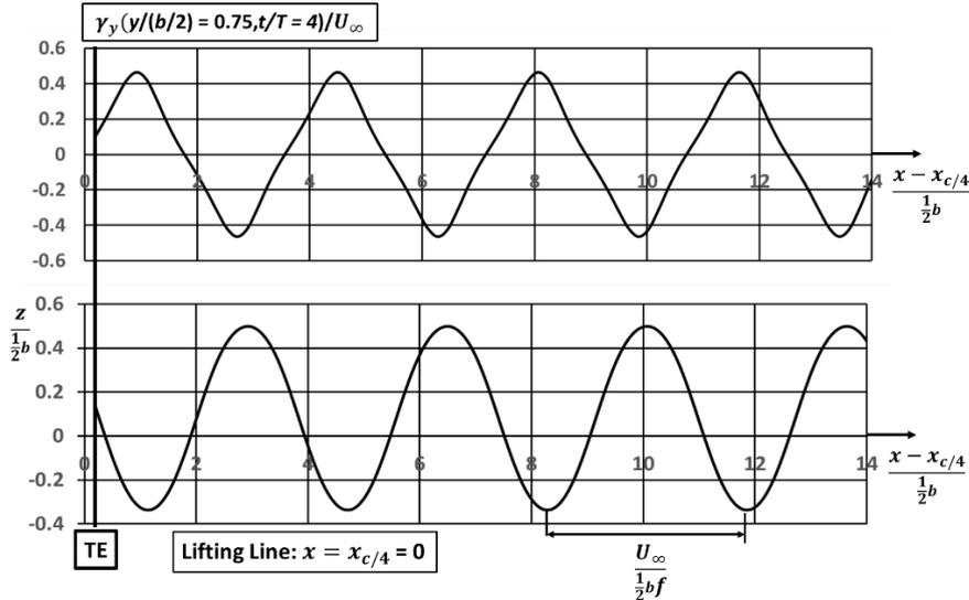
Figure 18 - Top: snapshot at  $t/T = 4$  of distribution spanwise component  $\gamma_y(y/(0.5b), t)/U_\infty$  vortex distribution along traverse  $y/(0.5b) = 0.75, z = 0$ , from trailing-edge to 14 semi-spans downstream. Bottom: estimate cross-section wake vortex sheet, at same instant, in plane  $y/(0.5b) = 0.75$ . Lifting-line model of simplified configuration, for the conditions listed in Tables 1 and 2,  $\theta_0 = 10$  deg,  $N = 80$ ,  $\frac{\Delta t}{T} = 0.05$ .
