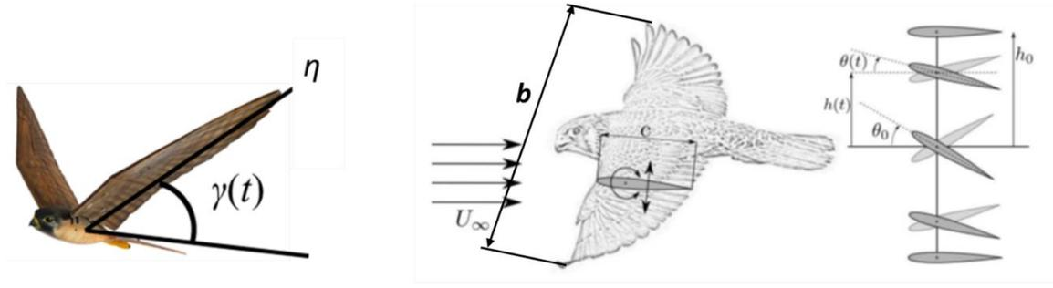
Figure 2 – Flapping/pitching motion of bird wings [13]. Left: definition flapping motion. Center Free stream and overall dimensions. Right: definition of equivalent 2D heaving/pitching motion airfoil sections.
