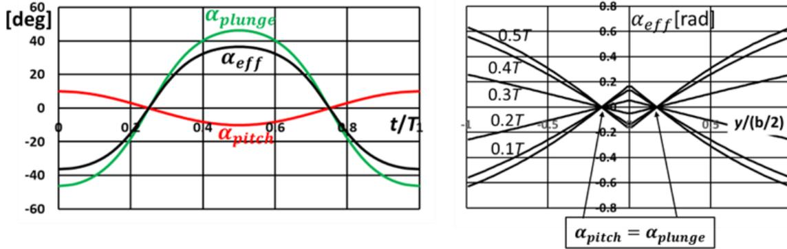
Figure 4 – Effective angle of attack  $\alpha_{eff}(y/0.5b, t/T)$  due to plunging/pitching motion. Left: as function of  $t/T$  at wing tips  $y/(b/2) = \pm 1$ . Right: as function of  $y/(b/2)$  at six moments during half a cycle, from upstroke  $t/T \in [0, 0.25]$  to downstroke  $t/T \in [0.25, 0.5]$ .  $\theta_1 = 0, \theta_0 = 10 \text{ deg}, \phi = 90 \text{ deg}, St = 0.3343$ .
