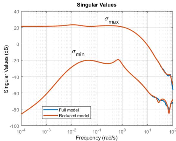
Figure 4 – Comparison between the maximum ( $\sigma_{max}$ ) and minimum ( $\sigma_{min}$ ) singular values of both full-order and reduced-order linear models.
