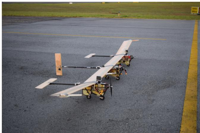
Figure 1 – X-HALE with four-meter-span configuration.
