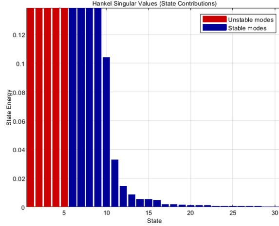
Figure 3 – Analysis of the stable and unstable modes using Hankel singular values.
