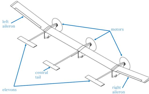
Figure 2 – Actuators description of the X-HALE with four-meter-span configuration.
