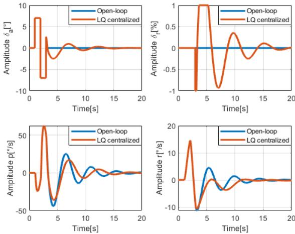
Figure 5 – Response to the 7-degree aileron doublet input (Centralized).
