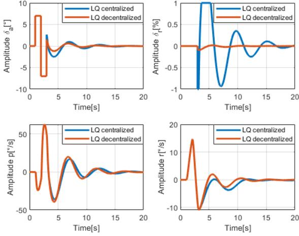
Figure 9 – Response to the 7-degree aileron doublet input.
