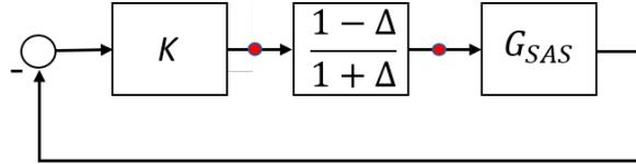
Figure 11 – Block diagram of the input disk margin concept.
