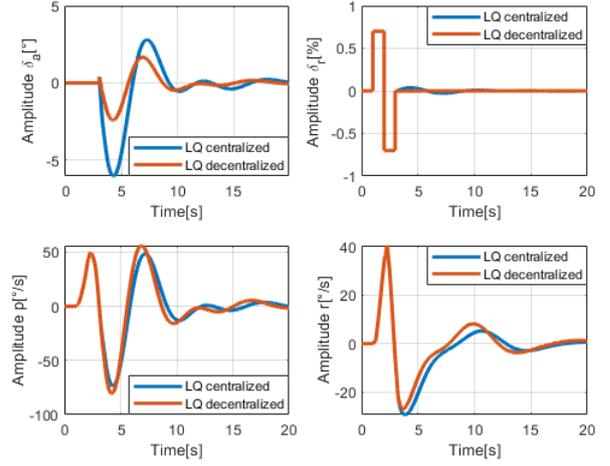
Figure 10 – Response to the 70-percent rudder doublet input.
