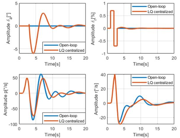
Figure 6 – Response to the 70-percent rudder doublet input (Centralized).
