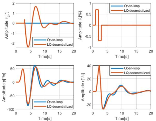
Figure 8 – Response to the 70-percent rudder doublet input (Decentralized).
