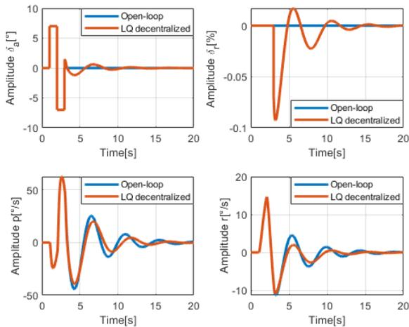
Figure 7 – Response to the 7-degree aileron doublet input (Decentralized).
