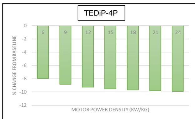
Figure 12. Change in trip fuel (%) over baseline for TEDiP-4P with increasing motor power density
