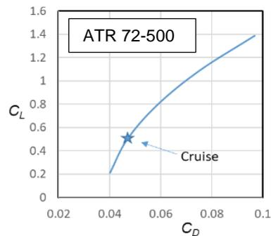
Figure 7. ATR 72-500 cruise drag polar using VSPAERO; 0.45 Mach number, 25,000 ft. altitude
