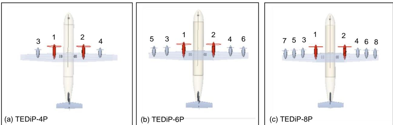
Figure 9. Three variants of ATR 72-500 with TEDiP systems
