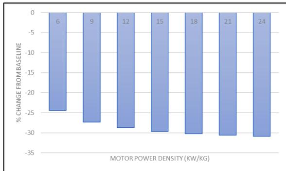
Figure 17. Change in TOFL (%) over baseline for TEDiP-8P with increasing motor power density
