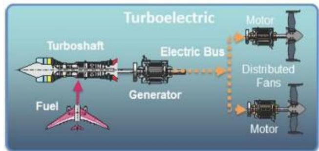
Figure 2. Turbo-electric architecture schematic [2]
