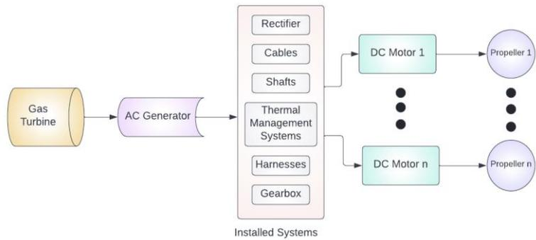
Figure 8. TEDiP system architecture
