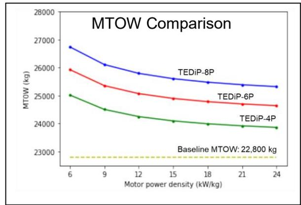
Figure 19. Change in MTOW for TEDiP variants with increasing motor power density
