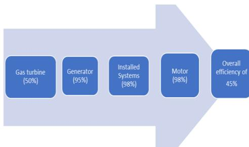
Figure 3(a). Schematic of turbo-electric system efficiency
