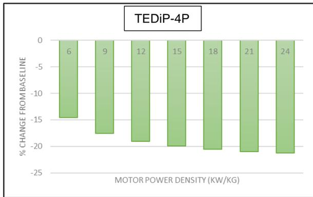
Figure 11. Change in TOFL (%) over baseline for TEDiP-4P with increasing motor power density
