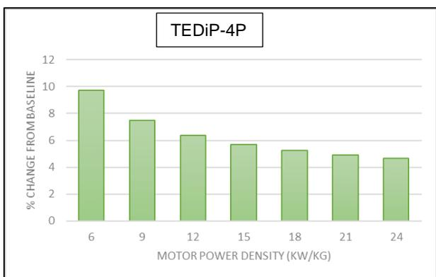
Table 3. Change in MTOW over baseline for TEDiP-4P with increasing motor power density
