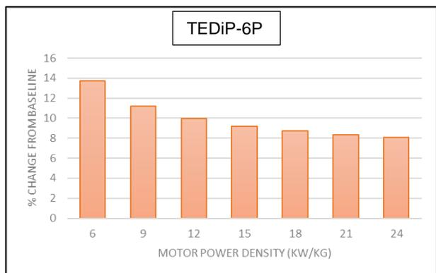
Figure 13. Change in MTOW (%) over baseline for TEDiP-6P with increasing motor power density
