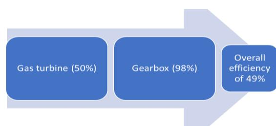
Figure 3(b). Schematic of turboprop efficiency
