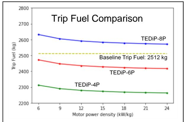
Figure 21. Change in trip fuel for TEDiP variants with increasing motor power density
