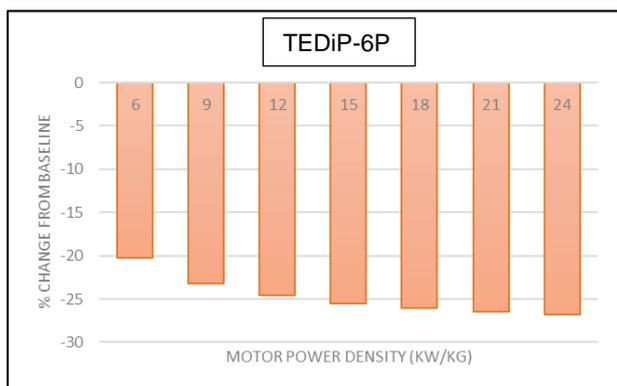
Figure 14. Change in TOFL (%) over baseline for TEDiP-6P with increasing motor power density
