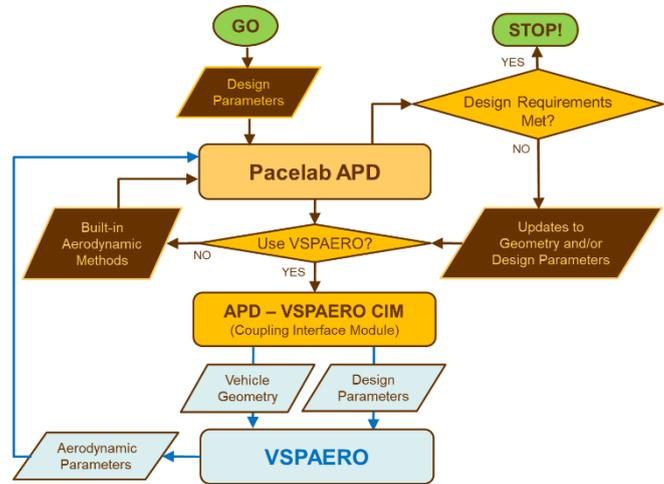
Figure 6. VSPAERO-Pacelab APD Coupling
