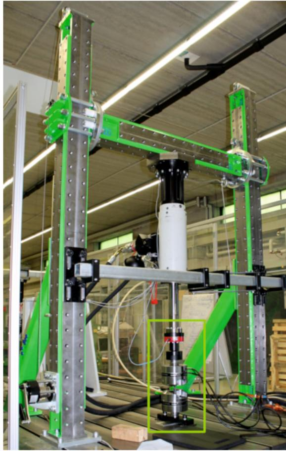
Figure 3 – Test rig with hydraulic cylinder.
