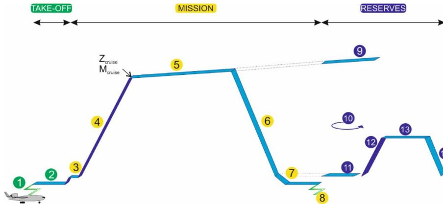
Figure 4 – Mission flight profile modeled with the Mission & Performance Module.
