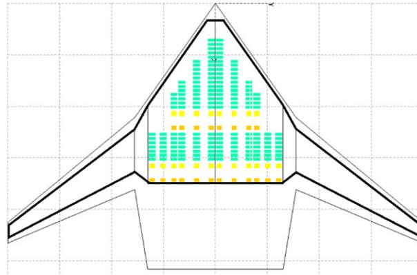
Figure 3 – Primary structure contours on a typical BWB configuration planform (top view).
