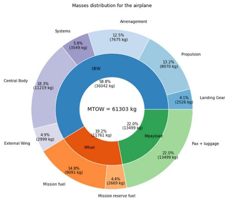
Figure 16 – SMILE configuration mass breakdown.
