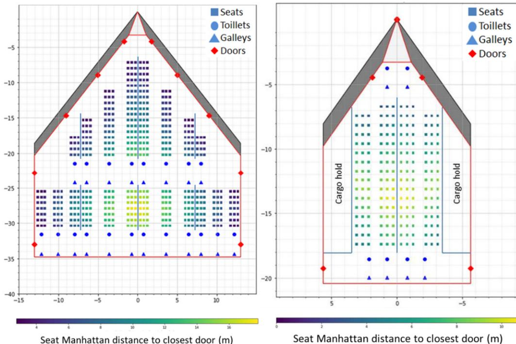
Figure 2 – Illustration of long-range (left) and short/medium-range (right) BWB passenger cabins.
