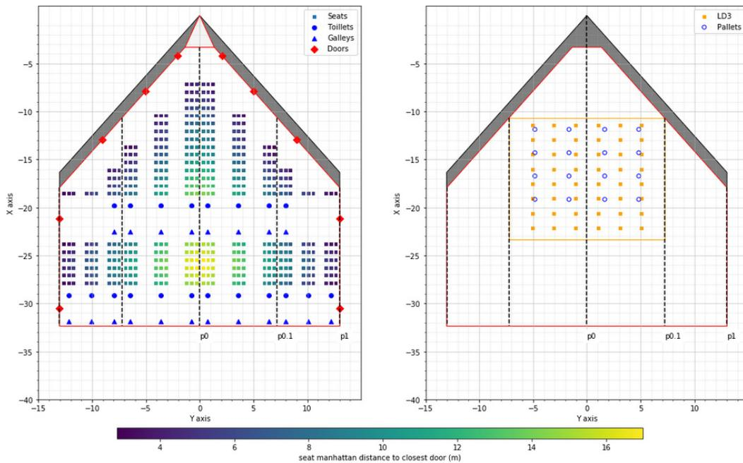
Figure 9 – BWB1 optimized configuration passenger cabin and cargo hold internal layout.
