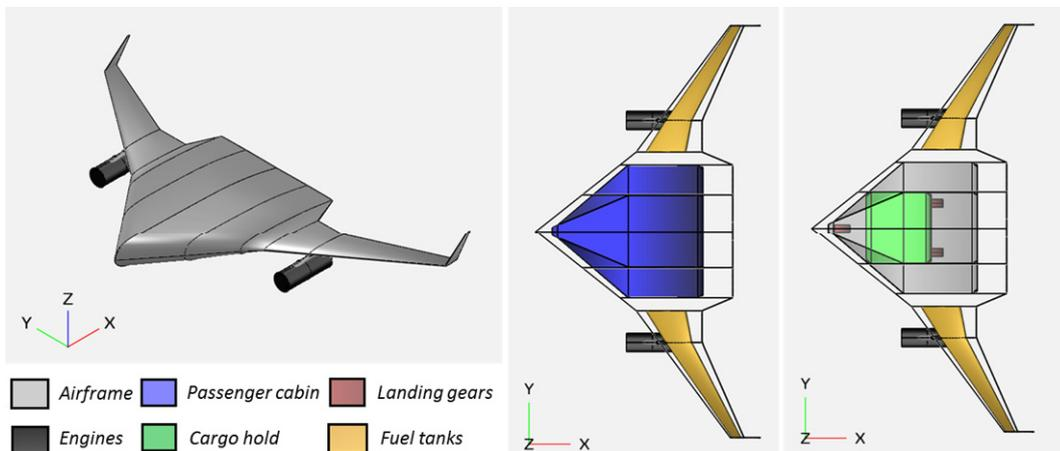
Figure 10 – BWB1 optimized configuration 3D view.
