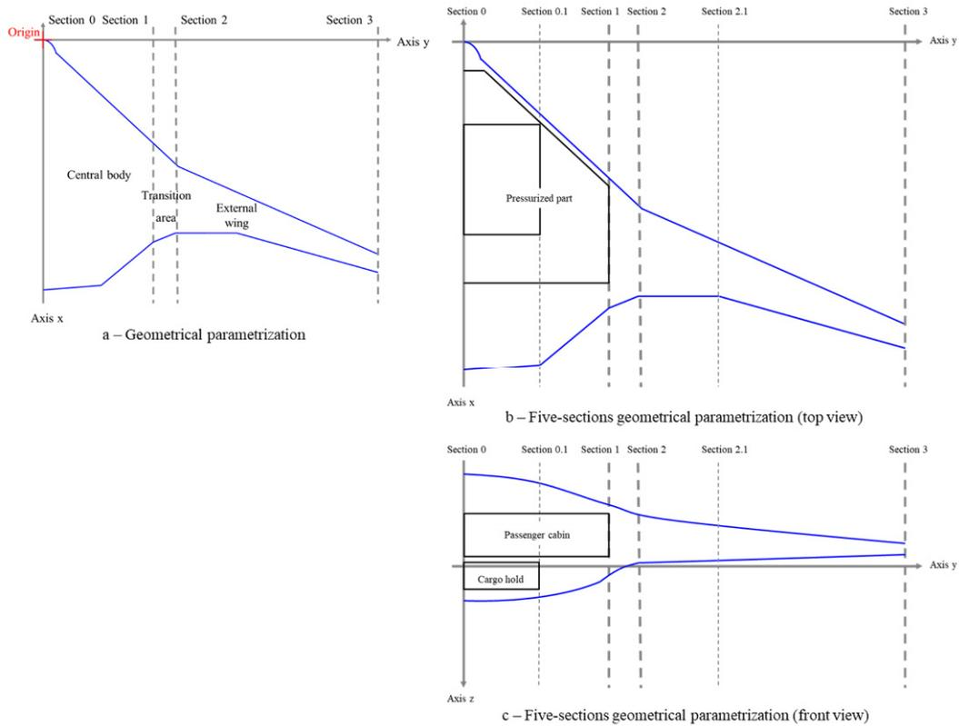
Figure 5 – Geometrical parameterization of the long-range BWB configurations.
