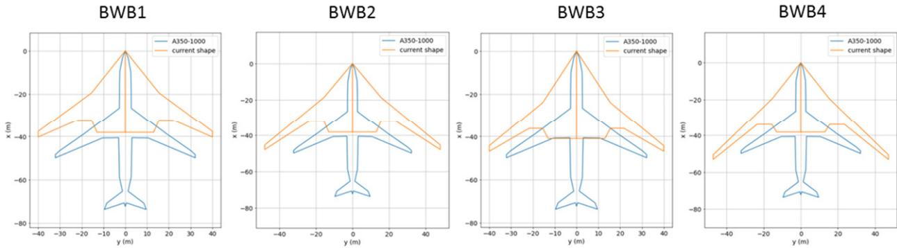
Figure 8 – Optimized BWB configurations planforms.
