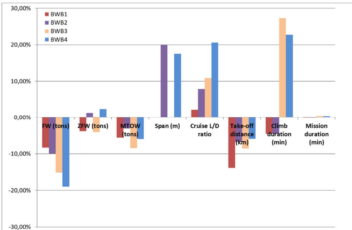
Figure 13 – Comparison of the optimized configurations with the reference configuration.
