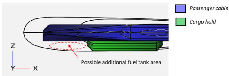
Figure 12 – Possible zone for an additional fuel tank in the front part of the central body.
