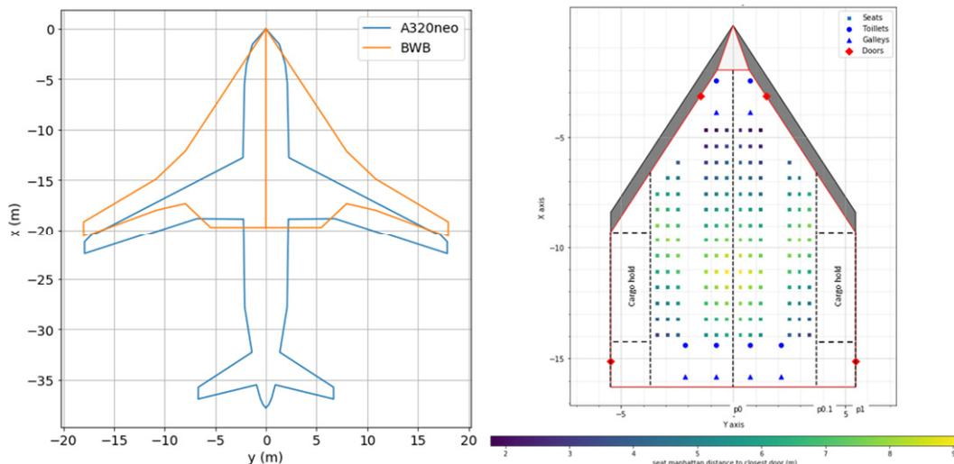
Figure 15 – SMILE configuration top view (left) and pressurized part internal layout (right).
