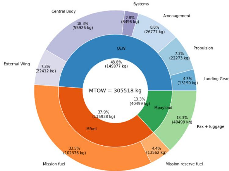
Figure 11 – BWB1 optimized configuration mass breakdown.
