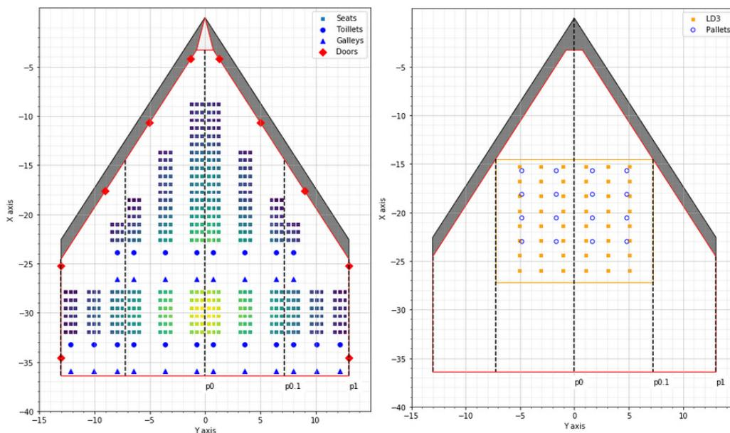
Figure 7 – Reference BWB configuration passenger cabin (left) and cargo hold (right) layout.
