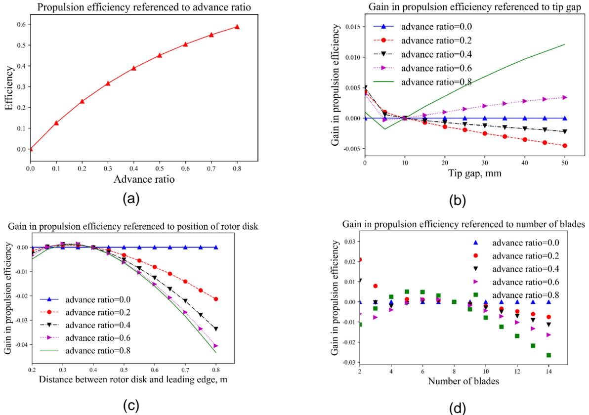
**Figure 4 Sensitivity study of propulsive efficiency depending on advance ratio, tip gap, distance between rotor disk and leading edge, number of blades**
