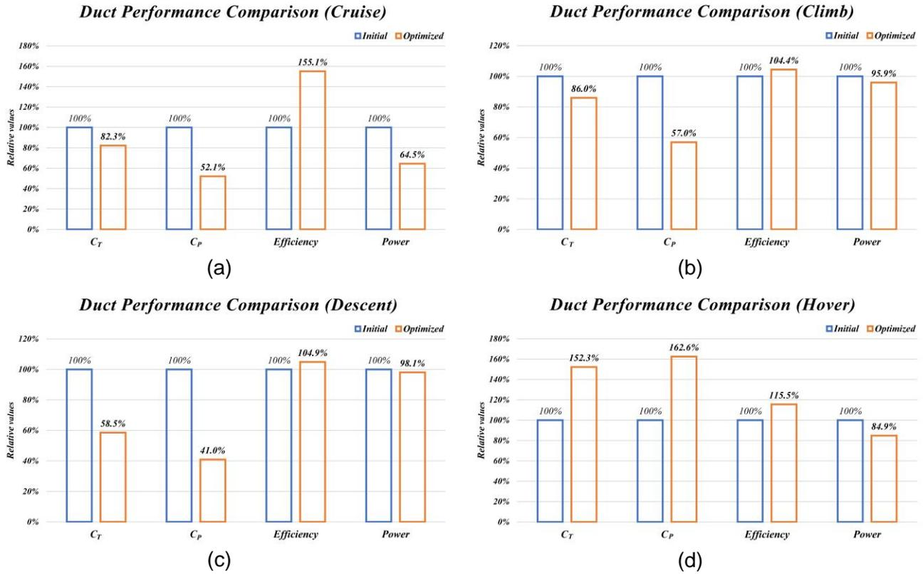
**Figure 7 Duct performance comparison in different scenario**
