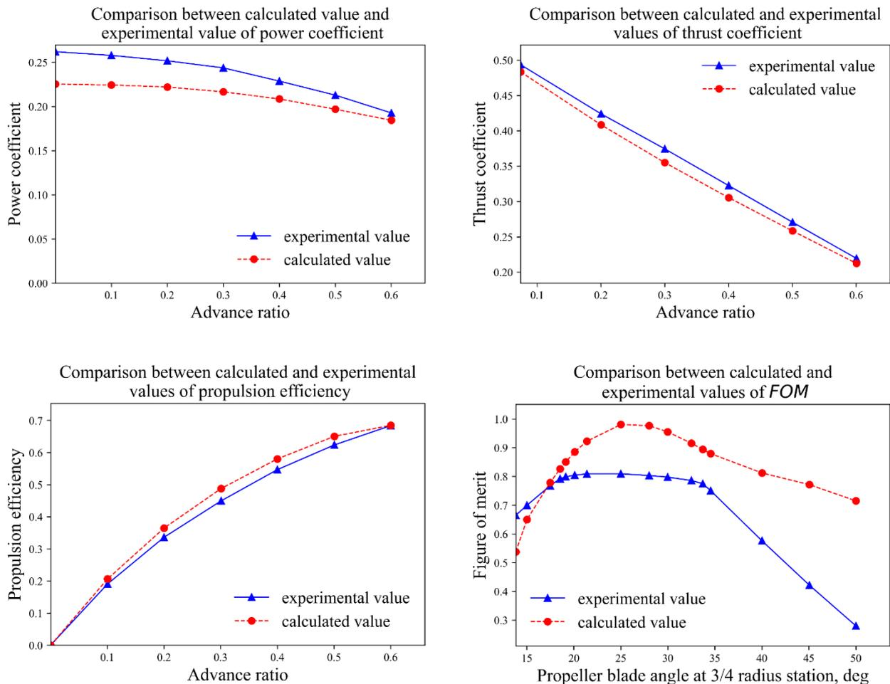
**Figure 2 Comparison of DFDC calculated results with wind tunnel experimental results**
