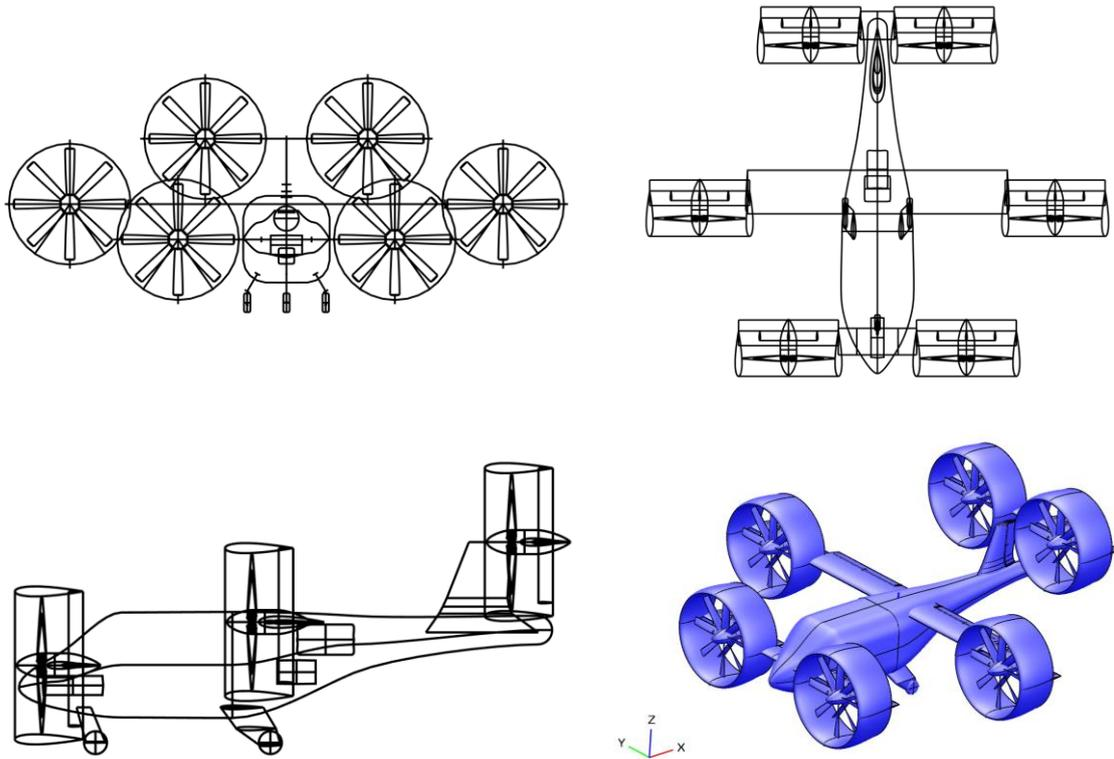
Figure 1 3-D views of NASA UAM tilt-duct eVTOL aircraft, reproduced with NASA OpenVSP, data based on Ref. [11]
