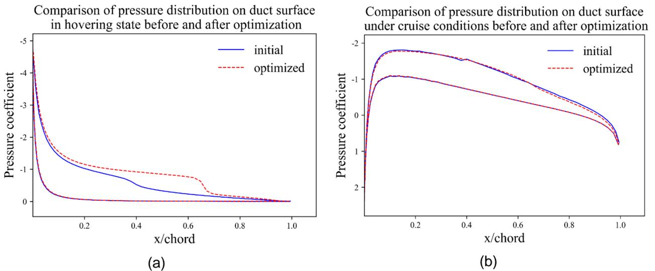
**Figure 8 Comparison of pressure distribution on duct surface in hovering and cruise state before and after optimization**
