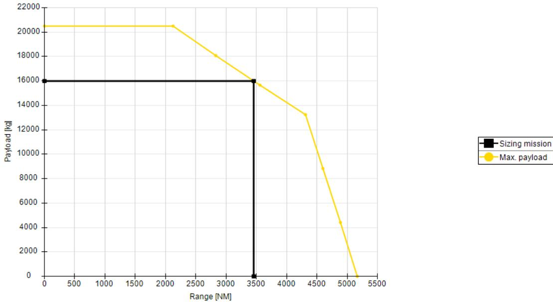
Fig. 3 SAFAM payload-range diagram
