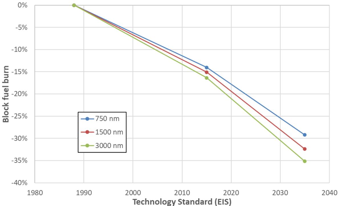
Figure 4 Fuel burn for progressive technology standards
