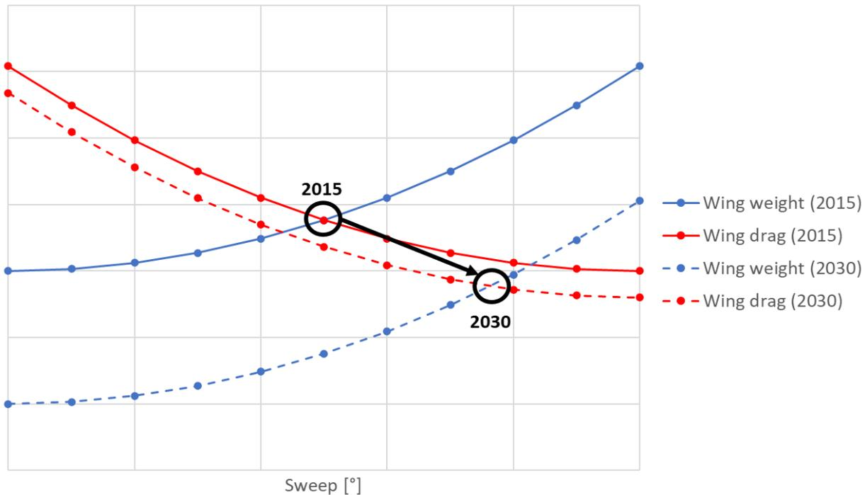
Figure 2 Effect of wing sweep on wing weight and drag for varying technology standards
